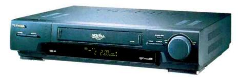
Toshiba's VHS Hi-Fi M-760 (\$550) uses six video heads to produce noise-free special effects and EP recordings that are said to be virtually indistinguishable from SP recordings.
