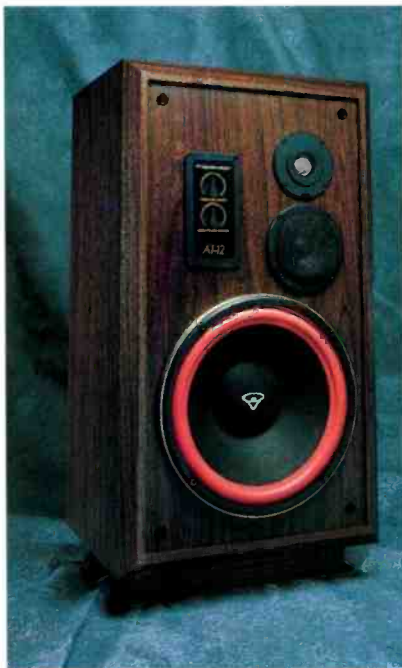
Cerwin-Vega's AT-12 ($690 a pair) is a three-way system with a 12-inch woofer and a 5-inch midrange driver. It's rated to handle 200 watts of power and has treble and midrange level controls. The 30-inch-tall cabinet is finished in woodgrain vinyl.
