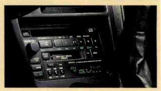
Bose sound system as standard equipment. Tight interior quarters limited the designers to only four loudspeakers: ported bass-reflex enclosures in the front doors with 4½-inch full-range drivers, a rearmounted 2½-inch Twiddler for the center channel (or cellular phone), and a ported-enclosure 4½-inch full-range driver in the firewall. The head unit is an Alpine cassette tuner. Maximum power is 165 watts, and a trunk-mounted six-disc CD changer can be added as an option.
