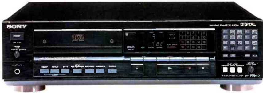
An optical transfer stage in Sony's top CD player, the CDP-705ESD, protects the audio circuits from noise generated in digital-to-analog conversion.
