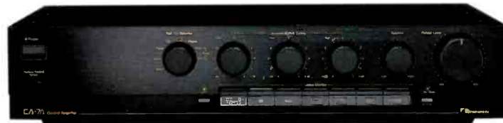
Nakamichi's remote-controlled CA-7A preamplifier isolates the control circuitry from the audio circuitry with extensive shielding and optical coupling.
