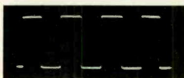
Figure 1. An actual photo of a square wave on an oscilloscope (top) will not show the vertical components of the waveform if the rise and fall times are fast enough. Some of the characteristics of a less-than-perfect square wave are shown in the drawing below.
