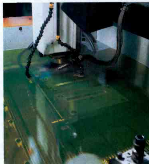
An electronic discharge machine, used by Paradigm to fabricate component molds
