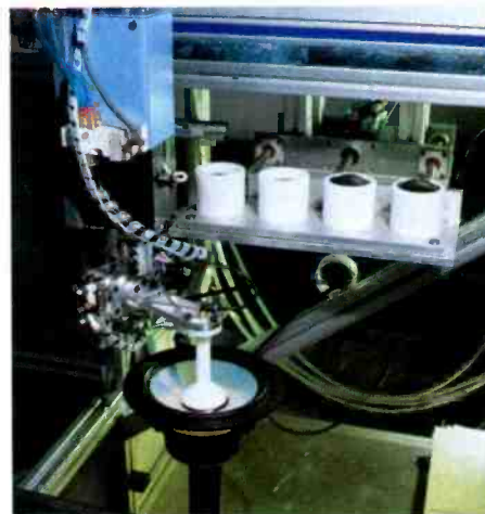
A robotic assembler glues a dustcap to a Paradigm woofer.
