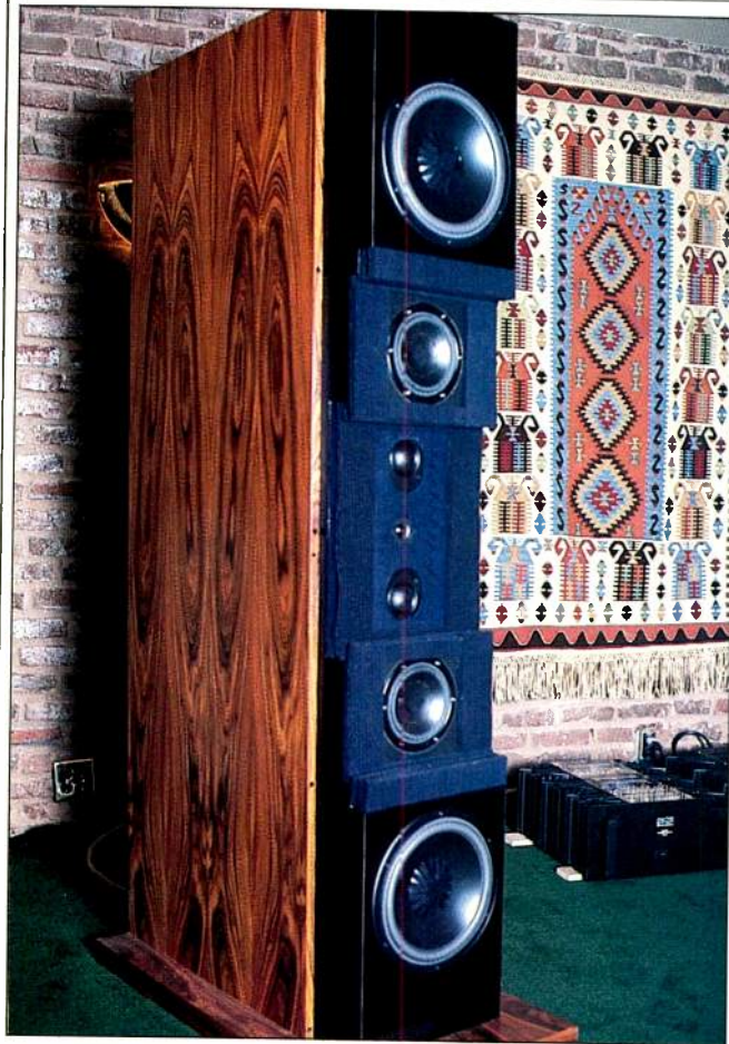
The seven drivers of the Duntech Sovereign 2001 are symmetrically mounted, top to bottom, to maintain the symmetry of its radiation patterns at all frequencies.
