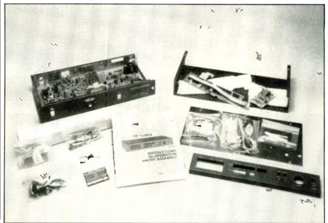
Following only 62 steps turns this kit into a finished tuner, thanks to pre-wired, pre-aligned circuit boards.
