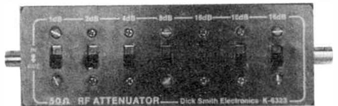
View of the completed attenuator box.
