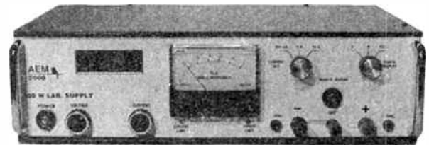
The unit is housed in an all-metal case, locally made by Horwood. The output terminals are 'floating', allowing either to be grounded in an external circuit connected to the supply.
