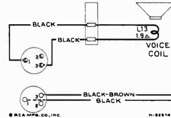
Figure 8—Loudspeaker Wiring
