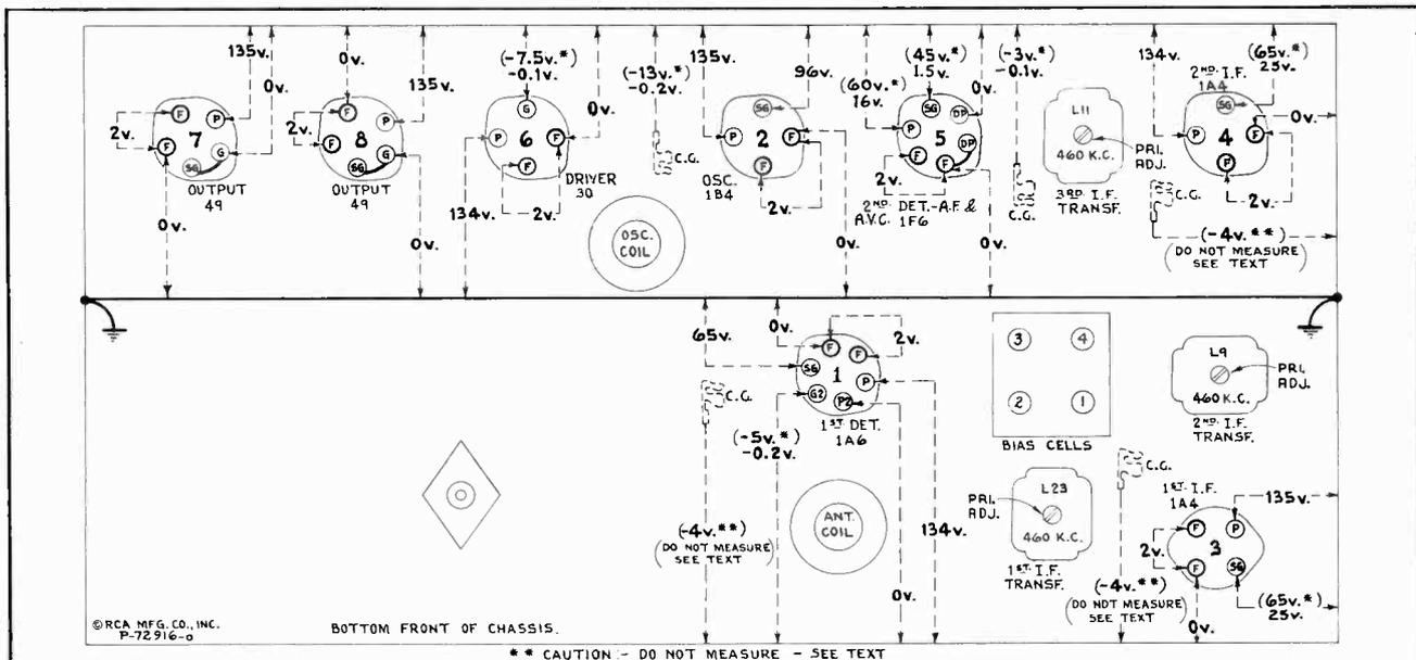
Figure 7—Radiotron Socket Voltages, Coil, and Trimmer Locations
