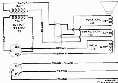
Figure 6—Loudspeaker Wiring
