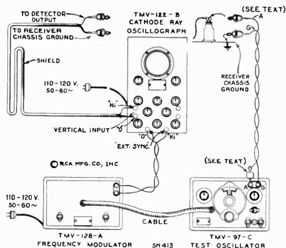
Figure 6—Alignment Apparatus Connections
