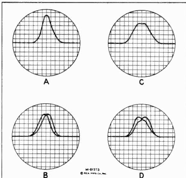
Figure 6—*I-F Alignment Oscillograph Curves*
