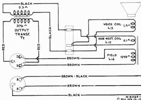
Figure 6—Loudspeaker Wiring
