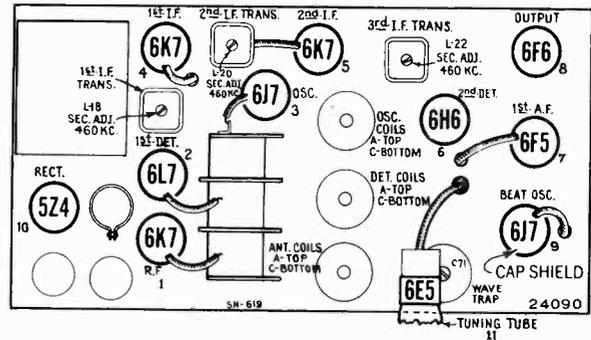
Figure 10—Radiotron and Coil Locations.
