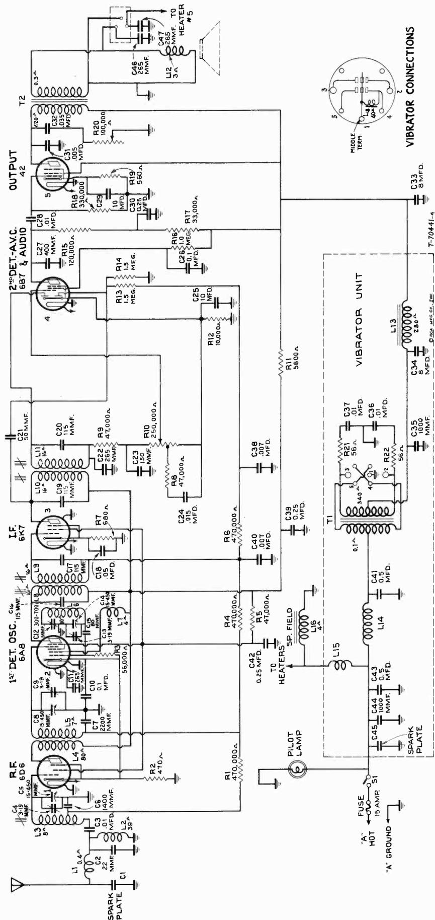
Figure 1—Schematic Circuit Diagram
