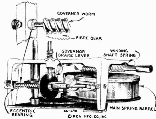
**Lubrication.**—All moving parts of the motor should be thoroughly cleaned and lubricated every six months to prevent excess wear and to assure proper operation. A small amount of grease should be applied to the worm gear of the governor, the gear of the winding shaft, and on the small pinion gear. All other points, including regulator friction pad, should be lubricated with light oil. All motor parts should be covered with a light film of oil to prevent rusting.
