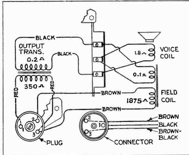
Figure 5—Loudspeaker Wiring
