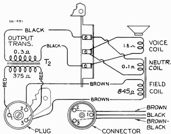
Figure 4—Loudspeaker Wiring
