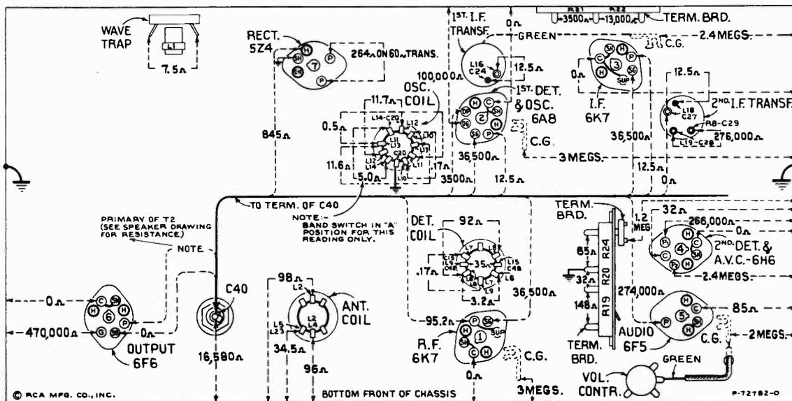
Figure 4—Resistance Diagram
