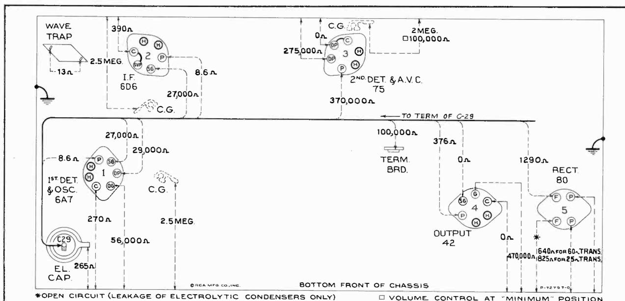
Figure 4—Resistance Diagram
