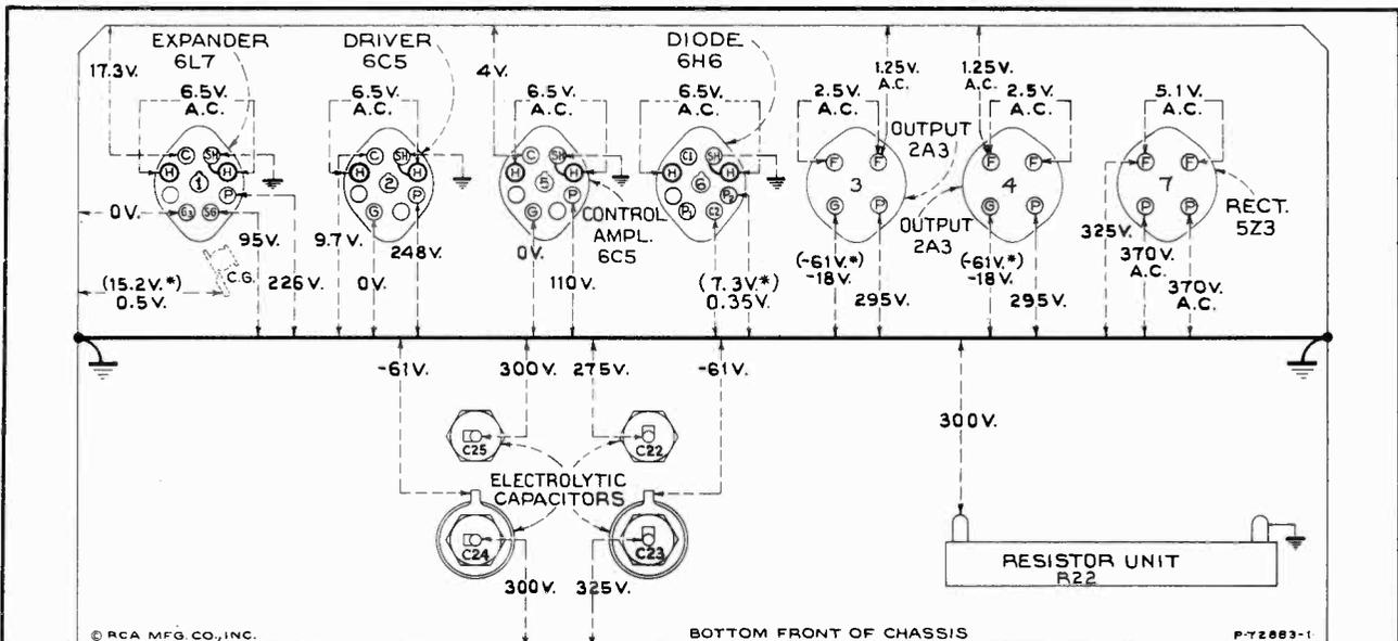
Figure 7—Radiotron Socket Voltages
