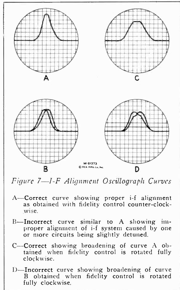
Figure 7—I-F Alignment Oscillograph Curves
