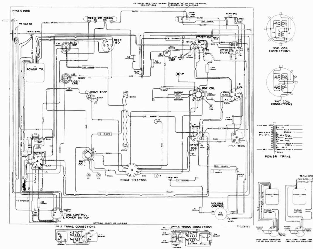
Figure 2—Chassis Wiring Diagram
