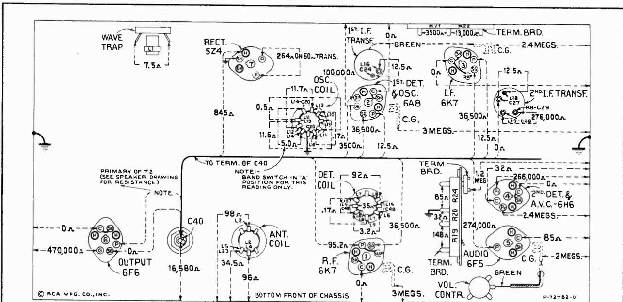
Figure 4—Resistance Diagram
