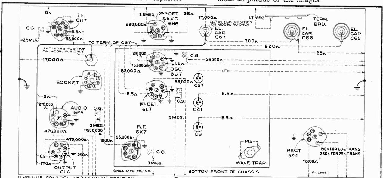
Figure 10—Resistance Diagram
