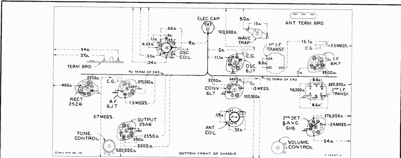
Figure 4—Resistance Diagram
