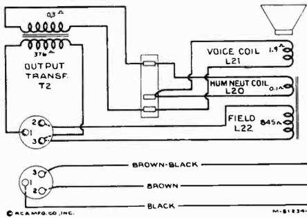
Figure 10—Loudspeaker Wiring
