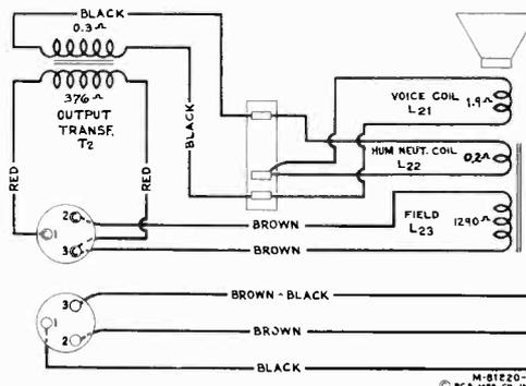
Figure 10—Loudspeaker Wiring
