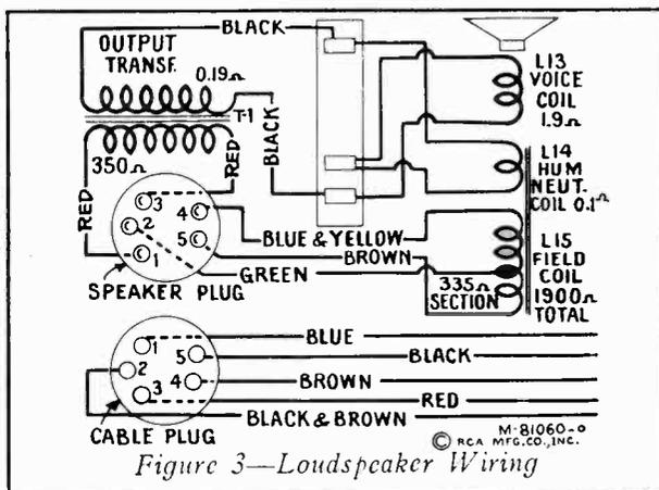
Figure 3—Loudspeaker Wiring
