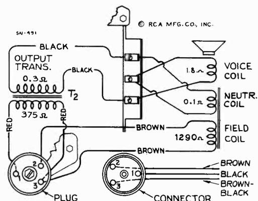
Figure 4—Loudspeaker Wiring
