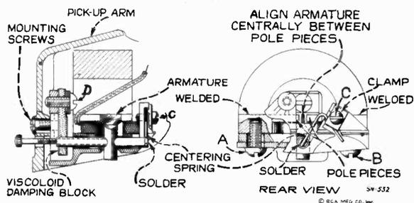
Figure 10—Details of Pickup
