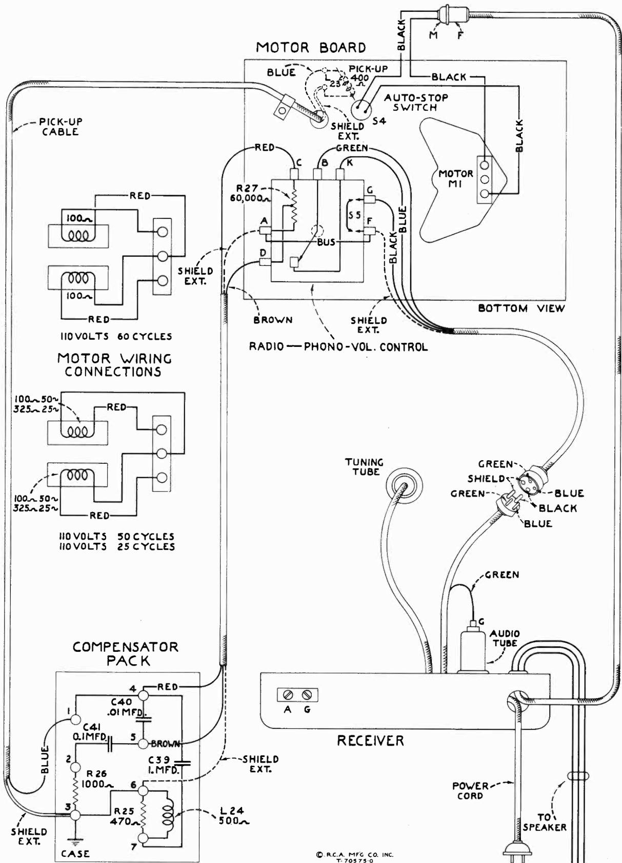
Figure 8—Assembly Wiring
