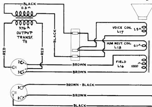
Figure 6—Loudspeaker Wiring
