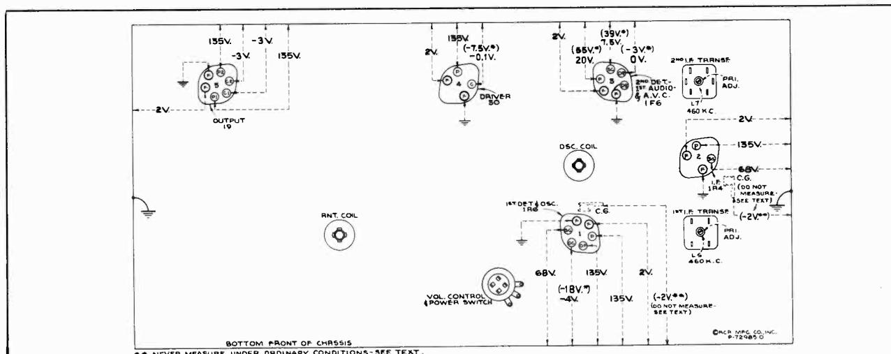
Figure 6—Radiotron Socket Voltages, Coil, and Trimmer Locations
