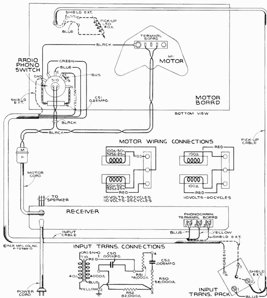
Figure 8—Assembly Wiring
