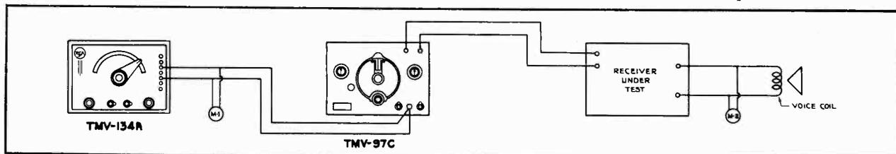
Figure 2—Receiver Fidelity Measurements
