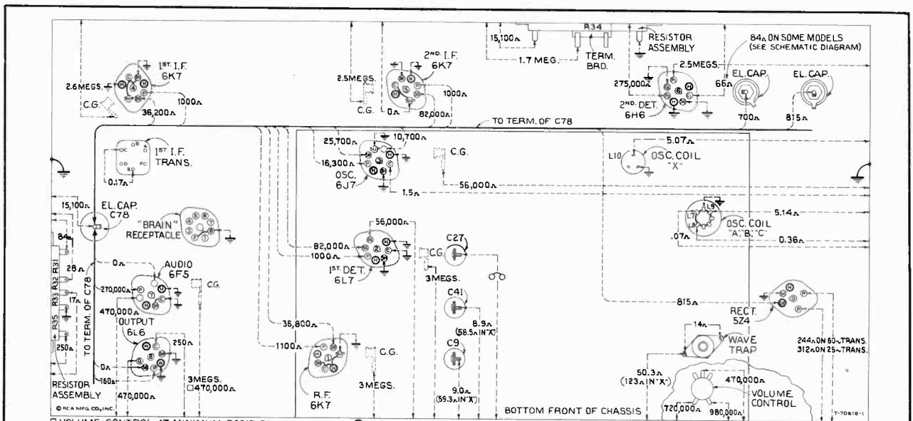
Figure 7—Resistance Diagram
