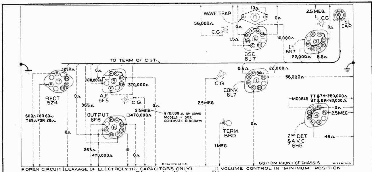
Figure 6—Resistance Diagram
