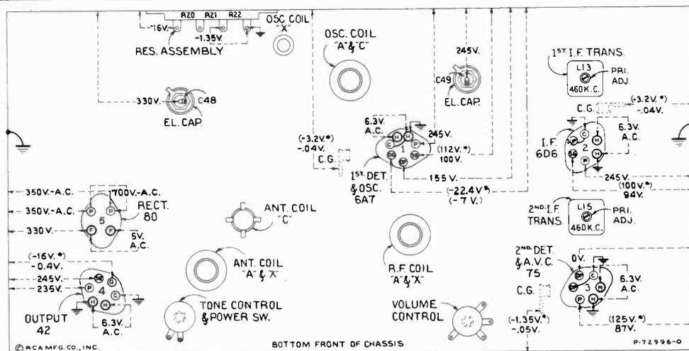
Figure 6—Radiotron Socket Voltages, Coil and Trimmer Locations
