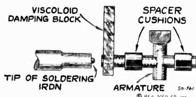
Figure 9—Special Soldering-Iron Tip
