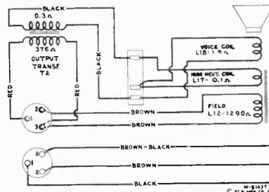
Figure 5—Loudspeaker Wiring
