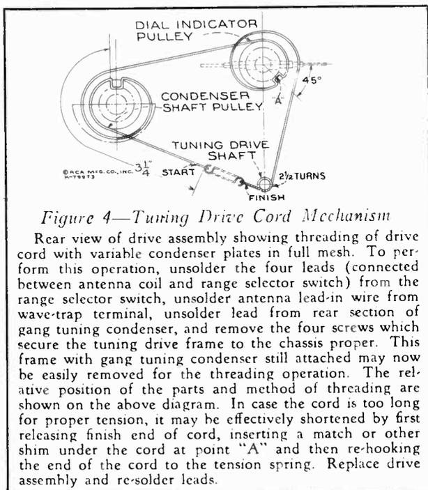
Figure 4—Tuning Drive Cord Mechanism
