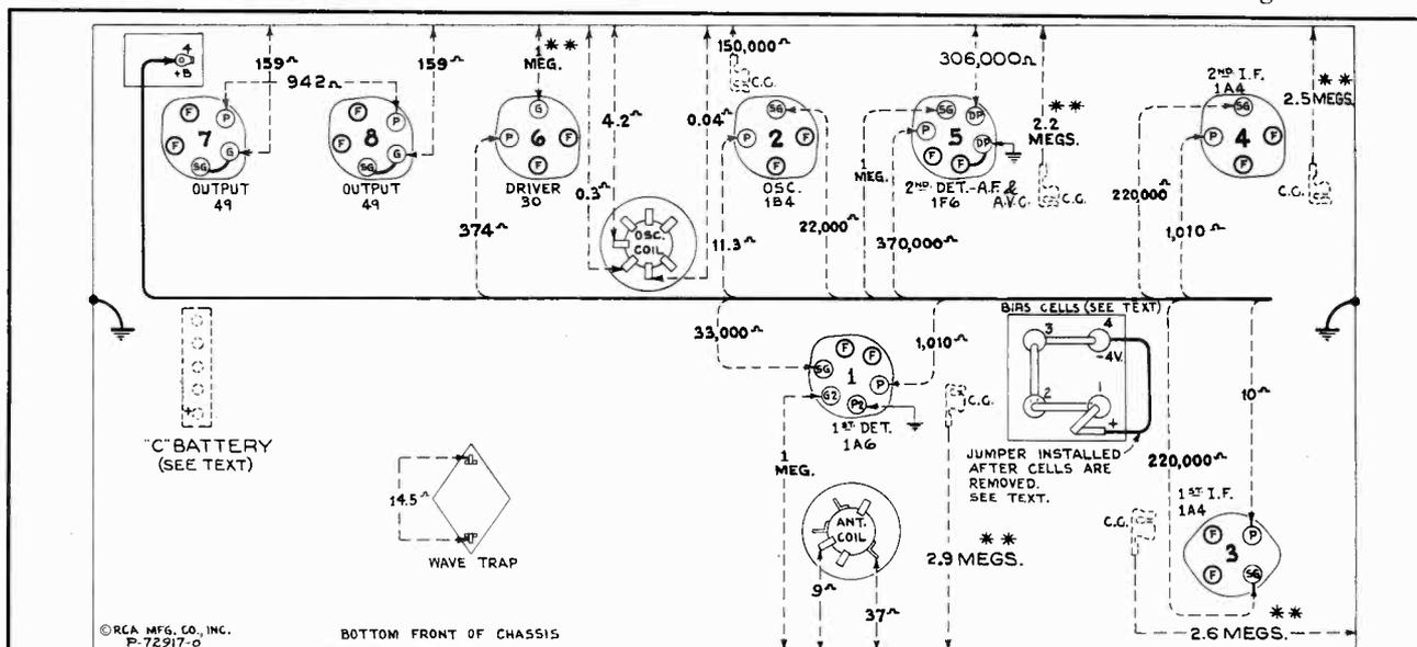
Figure 6—Resistance Diagram
