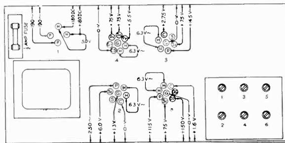
Figure 7—Tube Voltage Diagram
