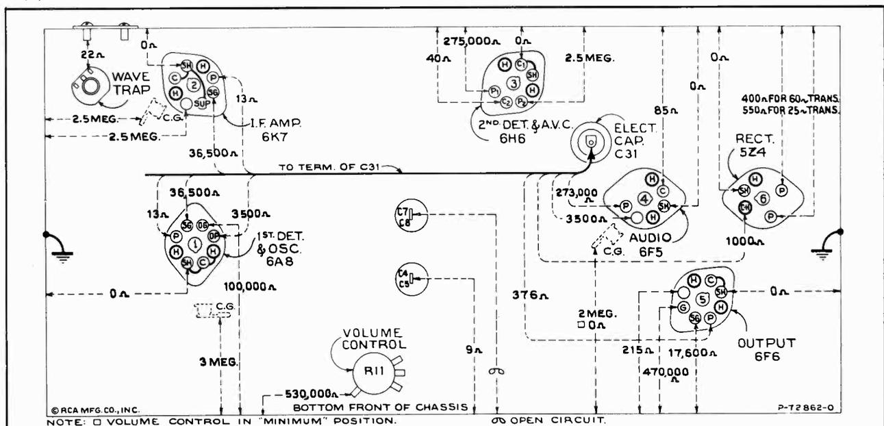
Figure 4—Resistance Diagram
