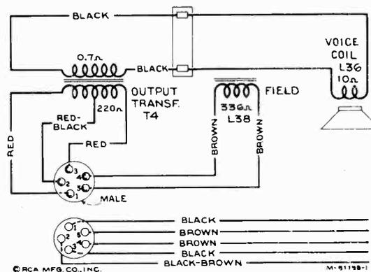
Figure 9—Loudspeaker Wiring
