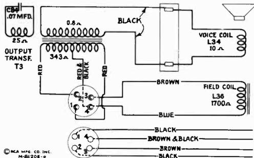
Figure 11—Loudspeaker Wiring
