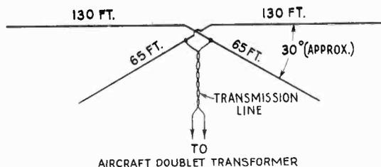
(c) Double Doublet Antenna for 160 and 80 Meter Bands
