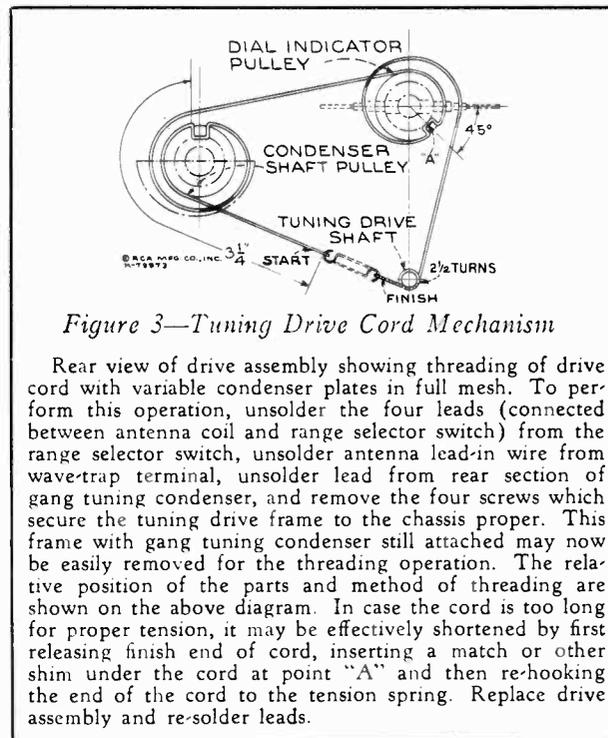
Figure 3—Tuning Drive Cord Mechanism
