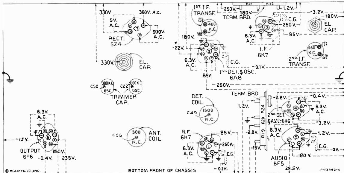
Figure 5—Radiotron Socket Voltages, Coil, and Trimmer Locations
