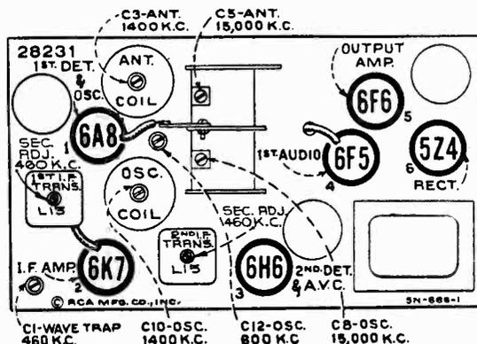
Figure 1—Radiotron, Coil, and Trimmer Locations
