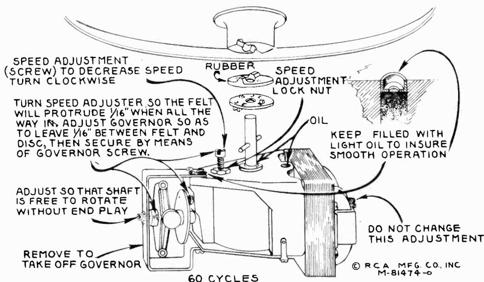
Figure 4—Details of 60-Cycle Motor
