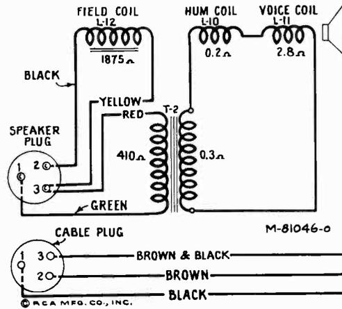
Figure 6—Loudspeaker Wiring
