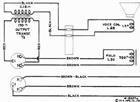
Figure 16—Loudspeaker Wiring
