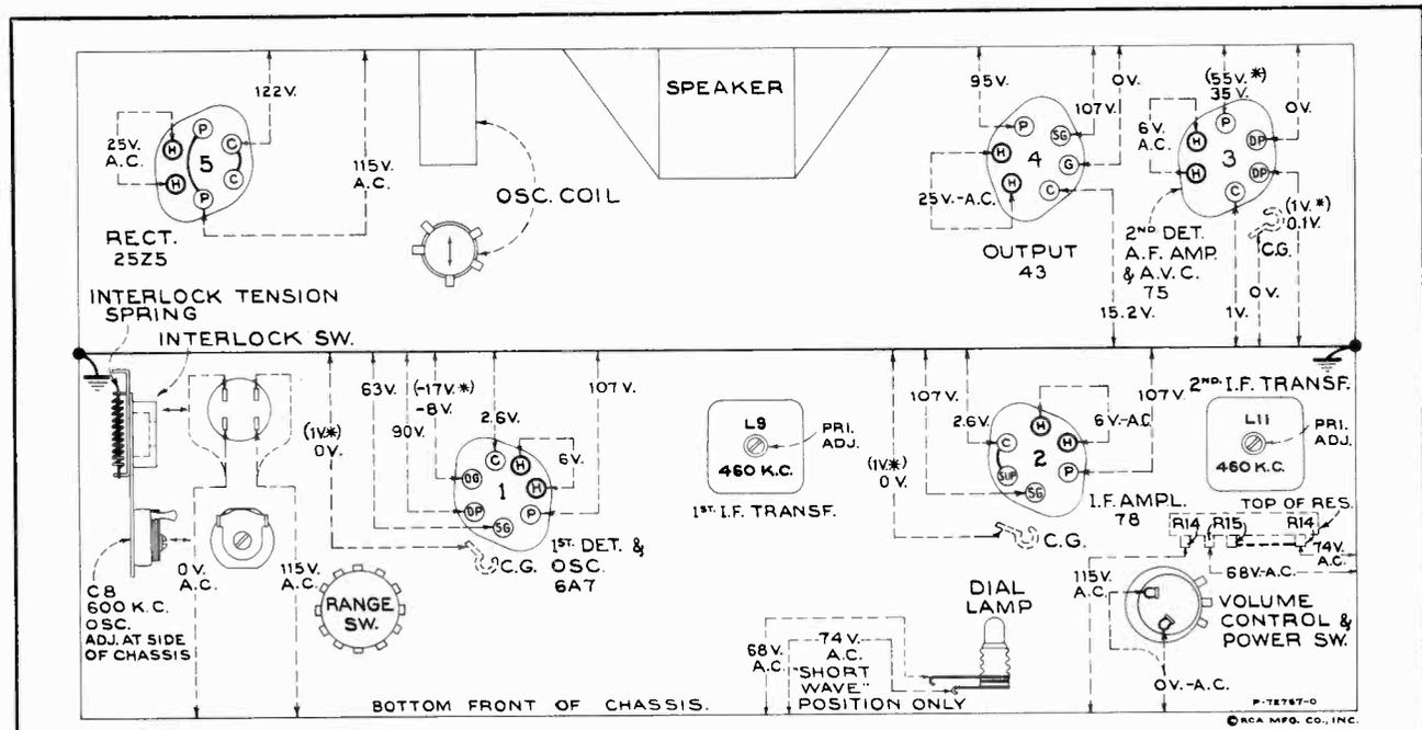
Figure 5—Radiotron Socket Voltages and Trimmer Locations
