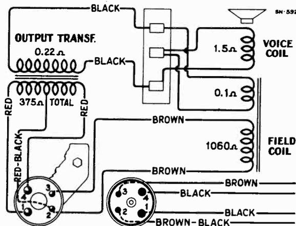
Figure 5—Loudspeaker Wiring
