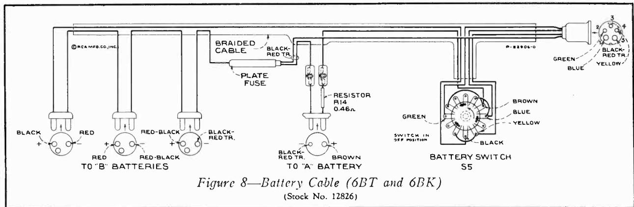
Figure 8—Battery Cable (6BT and 6BK)
