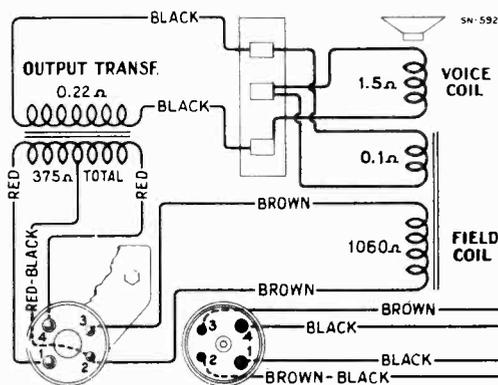
Figure 5—Loudspeaker Wiring
