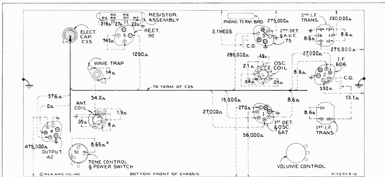
Figure 4—Resistance Diagram
