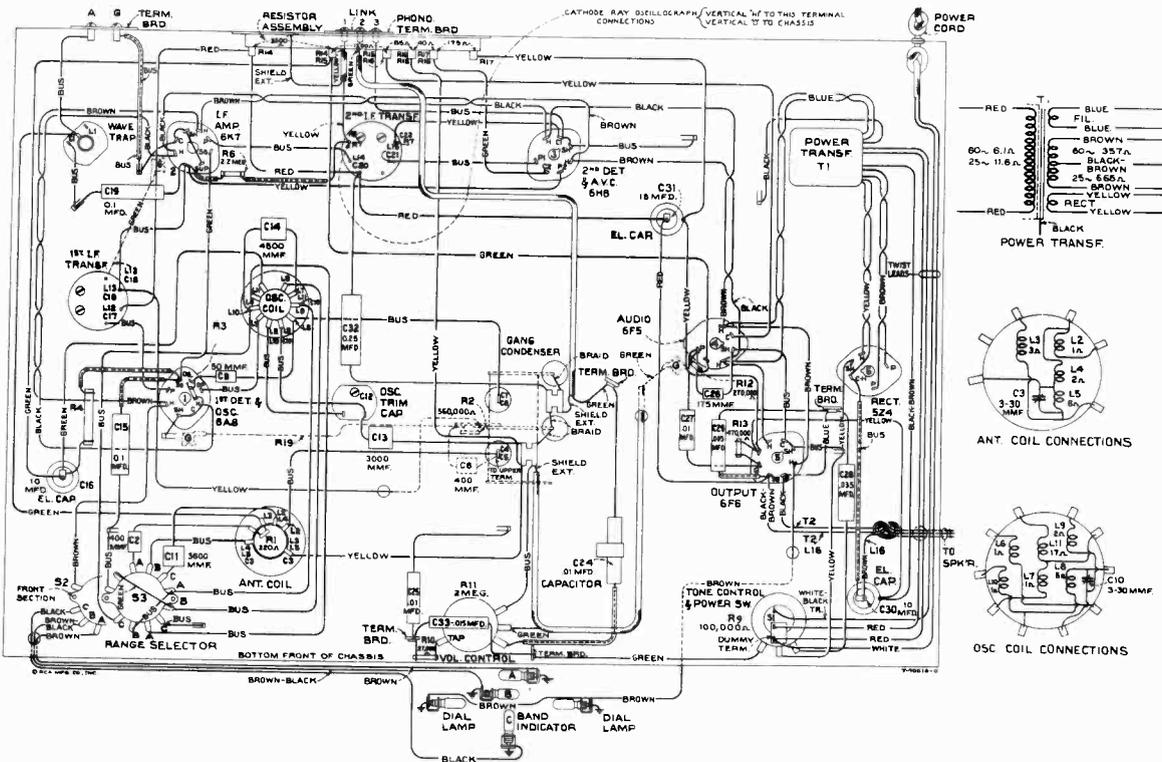
Figure 2—Chassis Wiring Diagram
