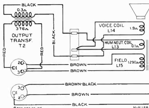
Figure 5—Loudspeaker Wiring
