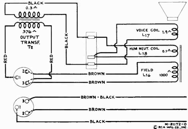
Figure 6—Loudspeaker Wiring
