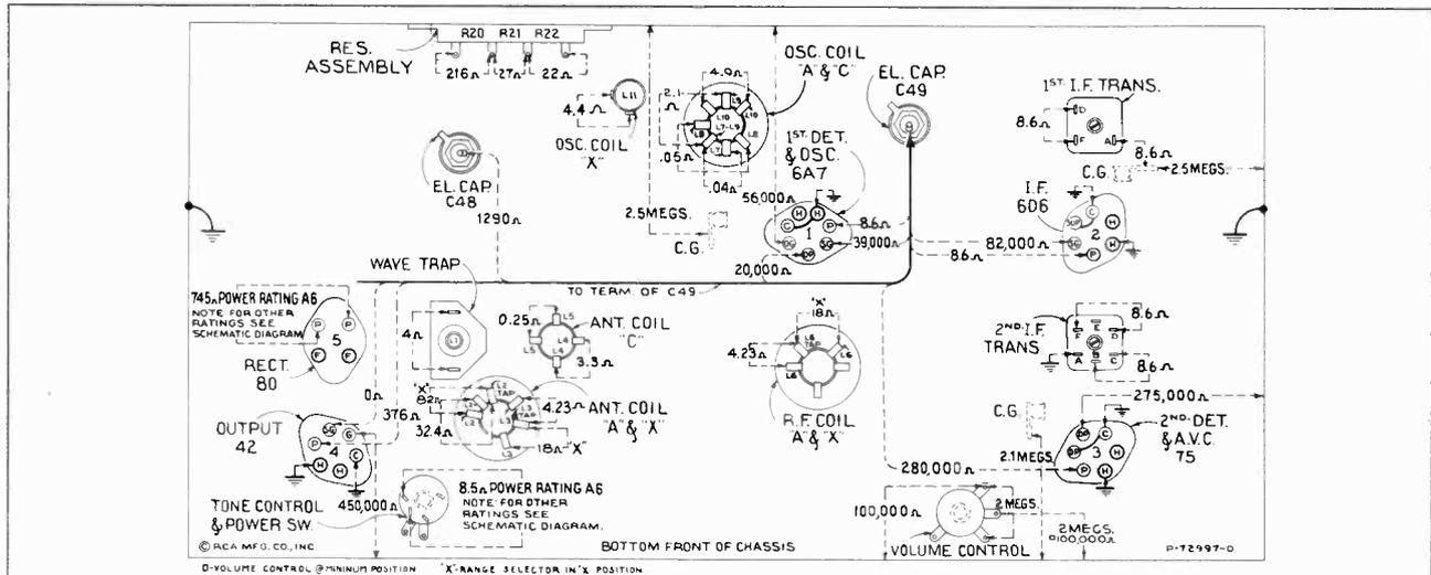
Figure 4—Resistance Diagram
