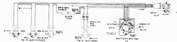
Figure 9—Battery Cable (8BT and 8BK)
