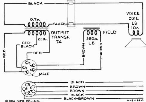
Figure 10—Loudspeaker Wiring
