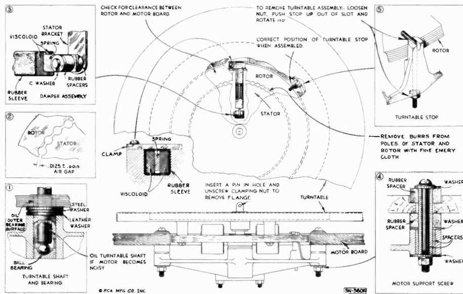
Figure 7—Details of Motor
