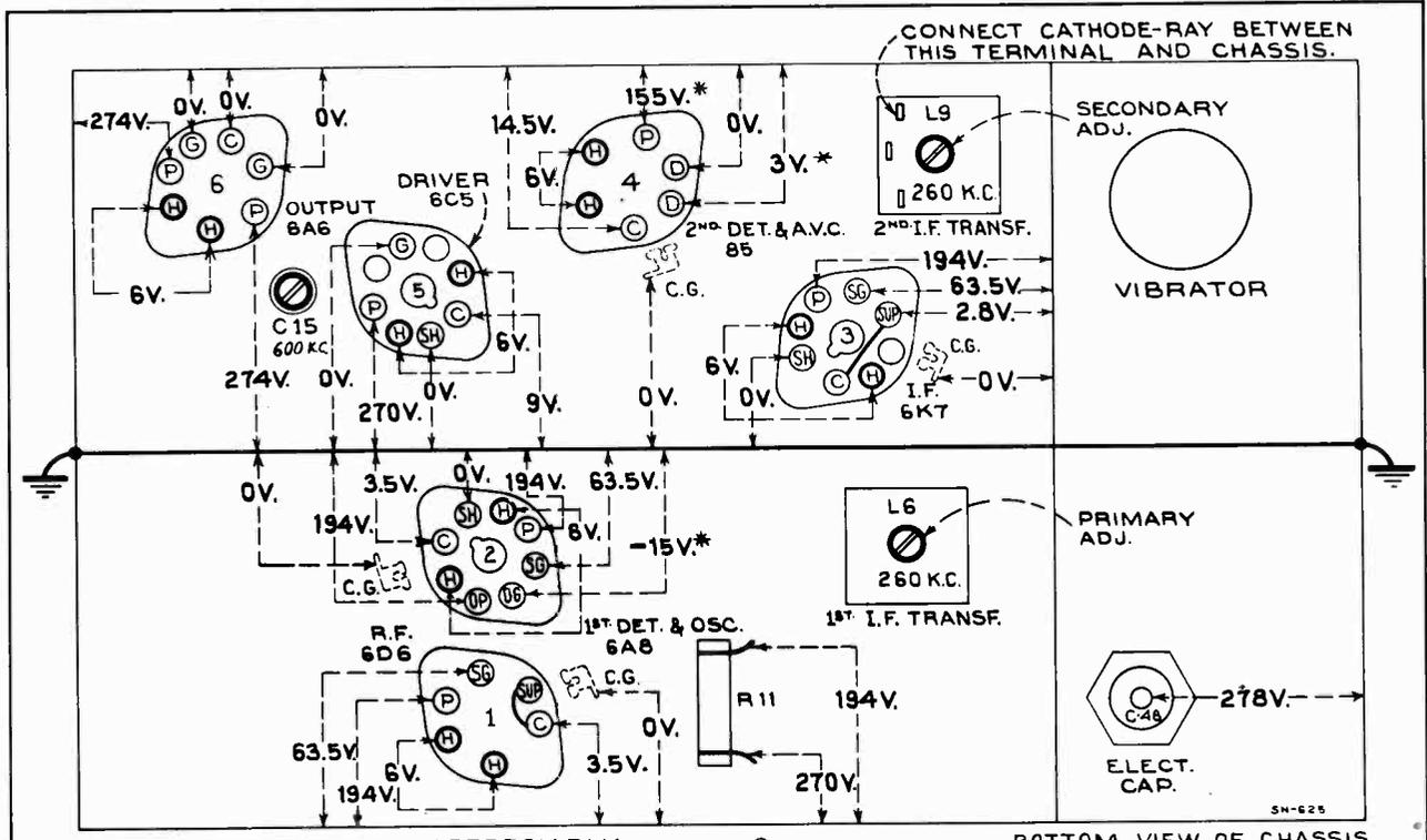
Figure 5—Radiotron Socket Voltages and Trimmer Locations
