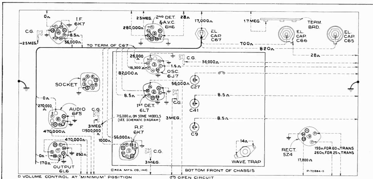
Figure 7—Resistance Diagram
