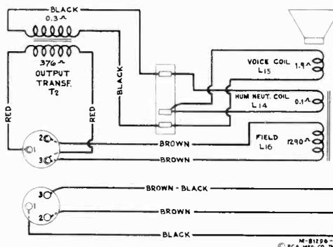
Figure 4—Loudspeaker Wiring
