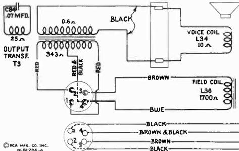
Figure 11—Loudspeaker Wiring
