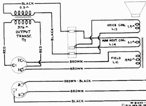
Figure 5—Loudspeaker Wiring
