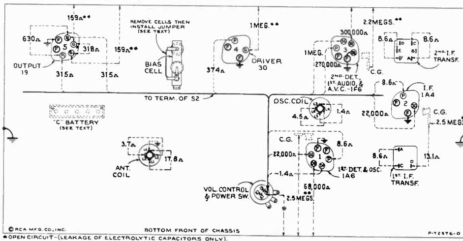
Figure 4—Resistance Diagram
