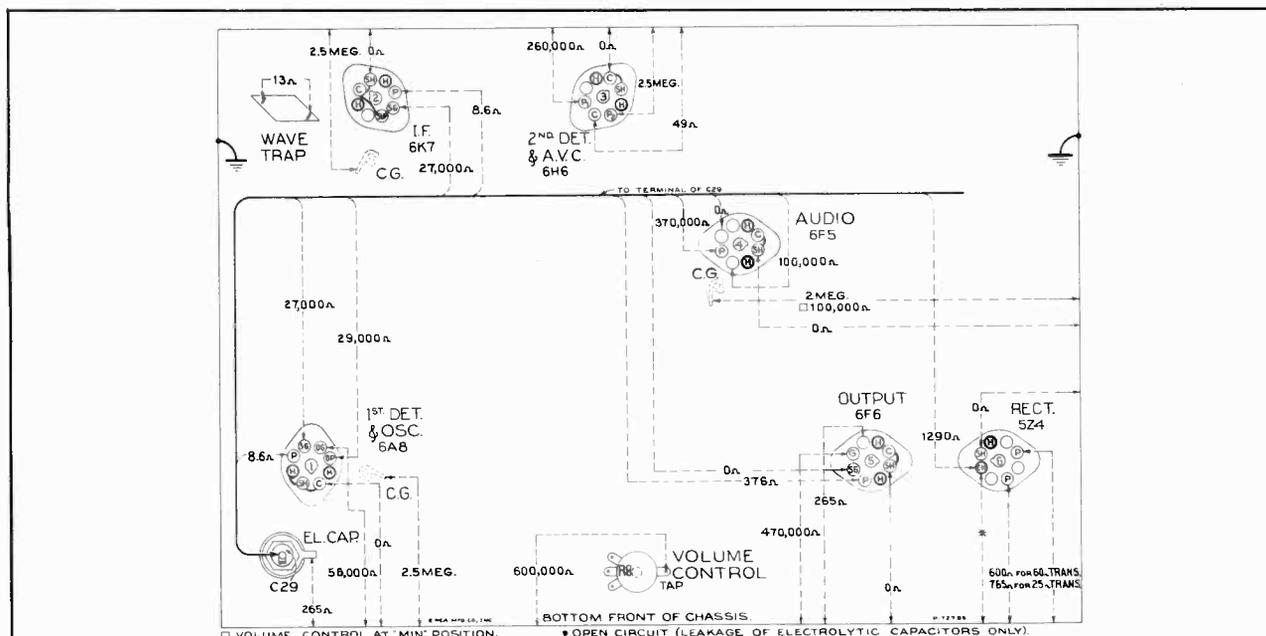
Figure 4—Resistance Diagram
