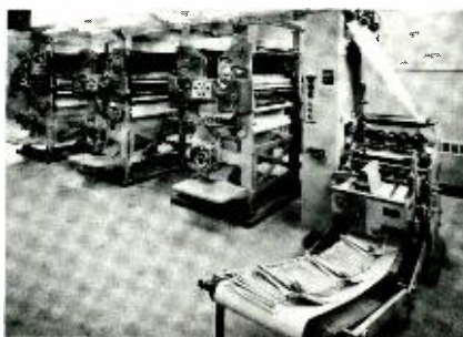
Fig. 9—A small community newspaper offset perfecting press. Each unit prints eight pages on the roll of paper held beneath. The dampening system is about eye level and the inking system at the top of each unit. The newspaper type folder is to the right. Courtesy, the Goss Co.
