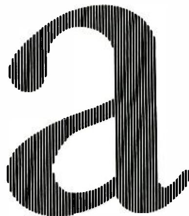
Fig. 3—Conceptual drawing of the formation of an “a” by vertical strokes.
