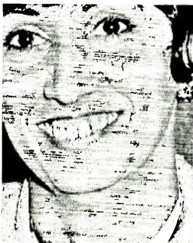
Fig. 12—An FM electronically screened halftone.
