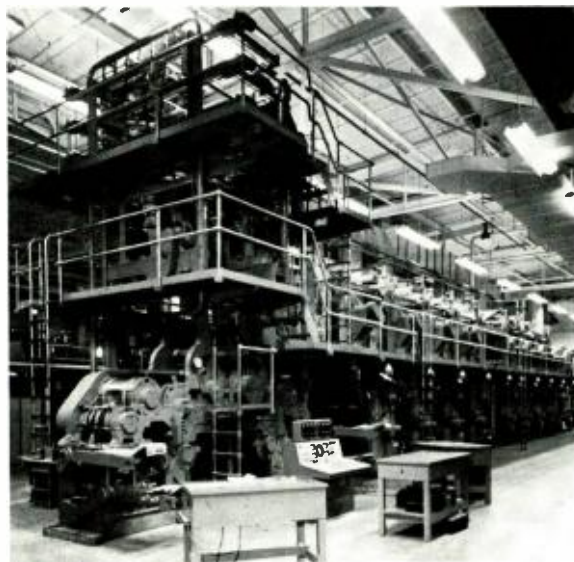
Fig. 11—An eight-unit rotogravure press with jaw type folder. This press produces four different 16-page signatures per revolution of the cylinder. Family Circle and Woman's Day are produced on this press. Courtesy John C. Motter Printing Press Co.
