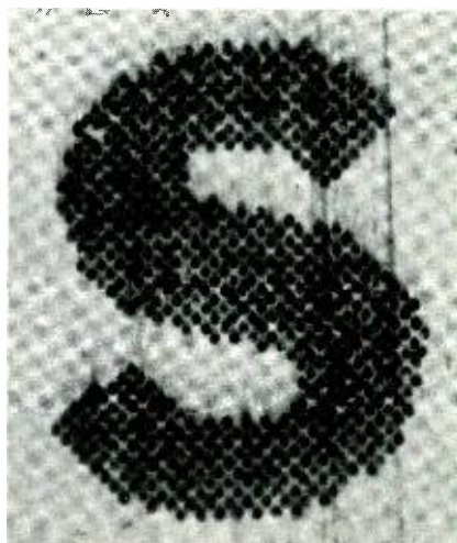
Fig. 6—Photomicrograph of printed results produced from laser engraved gravure cavities (12X magnification).
