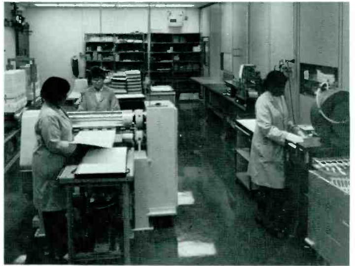
Fig. 3—Laminating and punching of alumina parts.
