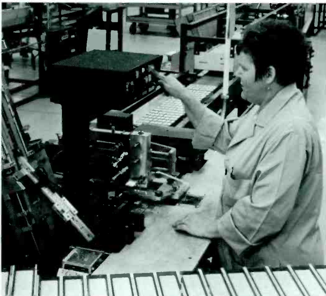
Fig. 6—Front end of screening machine—"magazine feed."
