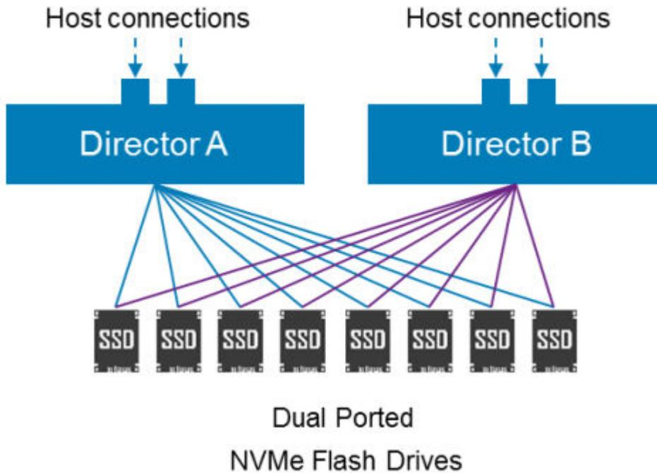
The use of Smart RAID on PowerMax provides customers with performance benefits, as both directors on an engine can drive I/O to all the flash drives. This creates balanced configurations in the system regardless of the number of RAID groups.
