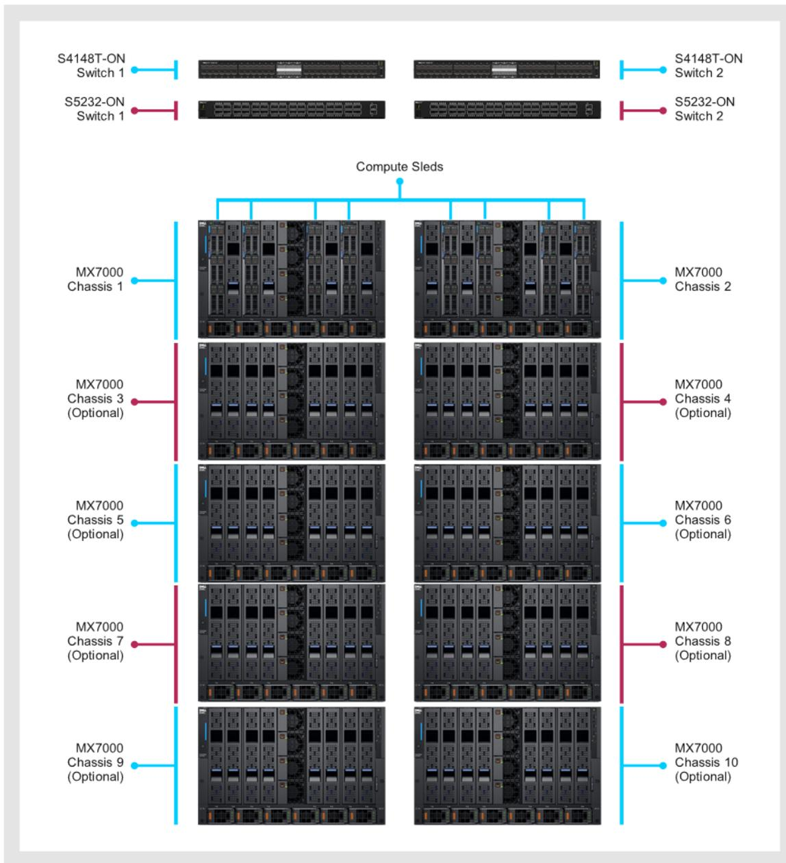
The compute domain in the example provides a total capacity of 80 two-CPU (MX740c) compute sleds.
