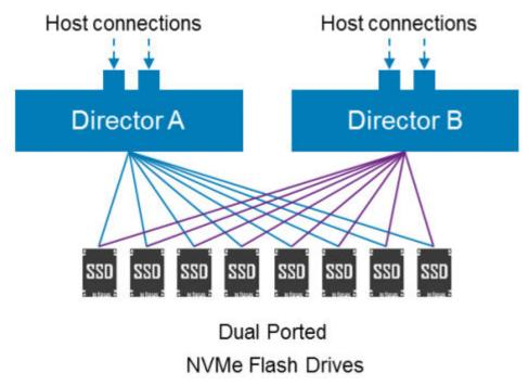
The use of Smart RAID on PowerMax provides customers with performance benefits, as both directors on an engine can drive I/O to all the flash drives. This creates balanced configurations in the system regardless of the number of RAID groups.
