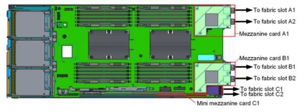
The following figure is an example of the MX740c mezzanine card slots.
