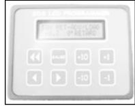
For RPM only ignition mapping (used mostly with naturally aspirated or race only engines), enter 0's for all the IGN RET/MAN PRESS values. This will subtract nothing from the RPM / IGN values.
