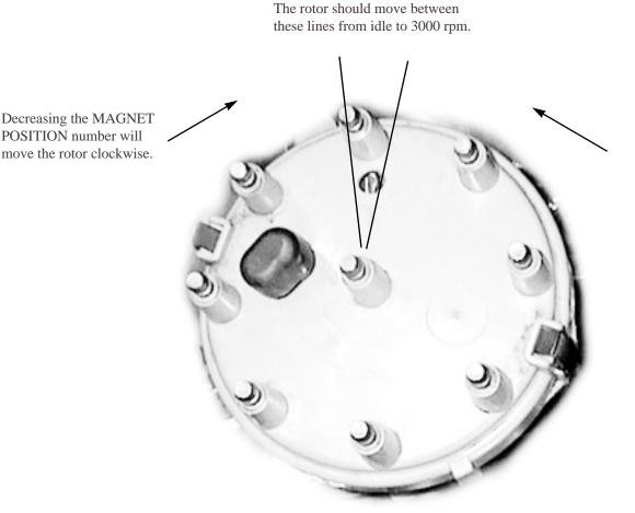
Increasing the MAGNET POSITION number will move the rotor counterclockwise.
