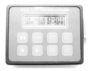
Scroll buttons for left '<', right '>' and fast '<<'.</li>Gauge button to go to gauge mode.Value change buttons for +10, -10, +1, and -1.
