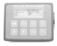
The MAGNET POSITION function on the SDS Programmer. Use the +1 and -1 buttons to adjust the value as described above.
