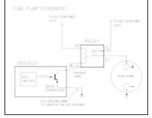
pin 30 to ignition switched 12 volts, be sure wire and power source will support the pump.
