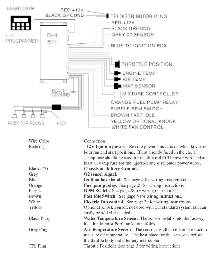
2. The TPS harness needs to be wired to the Ford throttle position sensor. A new plug is provided for this, cut the factory plug off the throttle body harness and crimp the supplied terminals to the wires. Insert the terminals into the supplied plug as follows:
