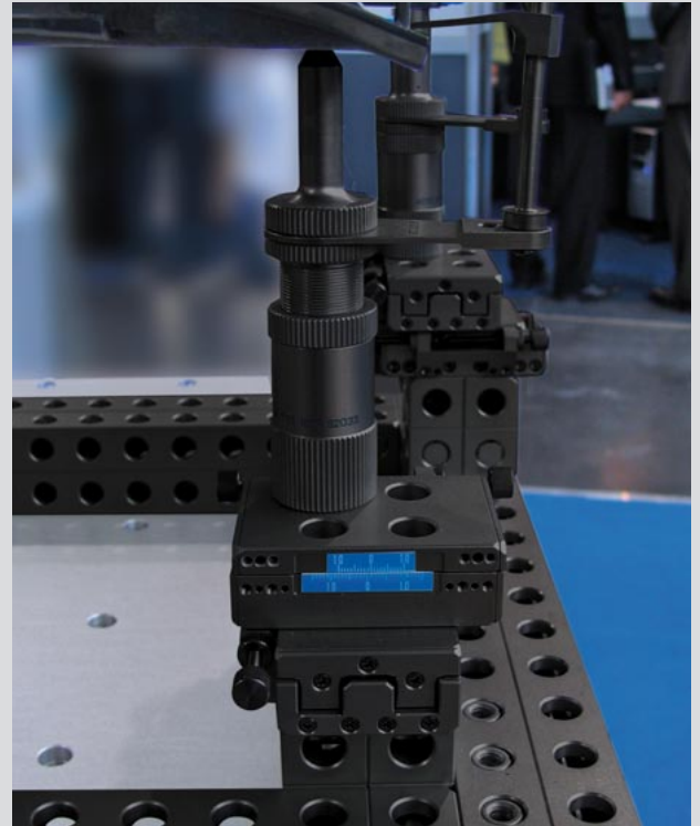
Above: The cross roller slide enables infinite adjustment of the center in the x and y axes - precise and reproducible using stop screws and scales with vernier.
