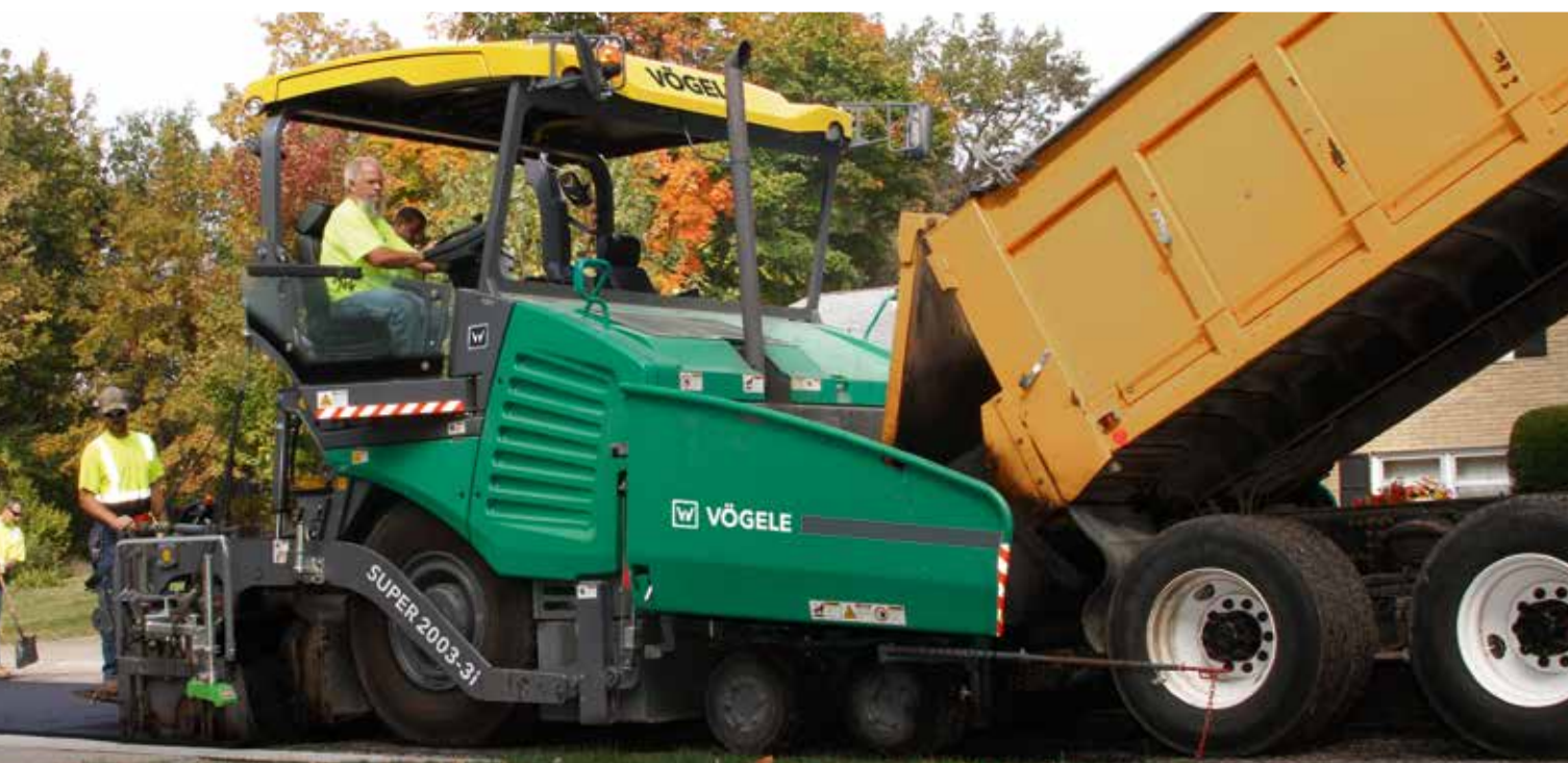
The power unit of the SUPER 2003-3i with diesel oxidation catalyst (DOC) and selective catalytic reduction (SCR) for exhaust gas after-treatment complies with the strict requirements of European exhaust emissions standard Stage 4 and US EPA standard Tier 4f.
