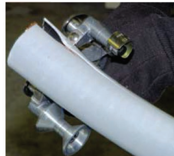
Teeth Gripping and Pulling Off Laminate Layer.
