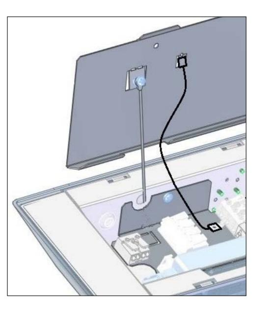
6. Air Control Remote Unit.. Unscrew the two srews to lift away the lid. The remote box is ready to be wired up.
