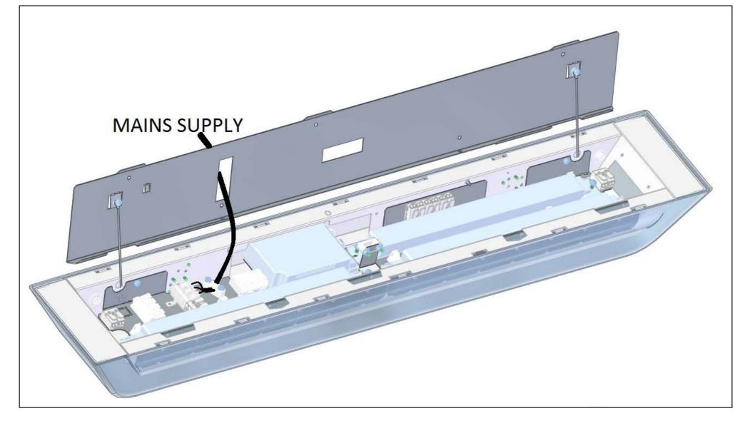
Mains Supply - 0.75mm<sup>2</sup> - 2.5mm<sup>2</sup>, Solid or Stranded mains rated.
