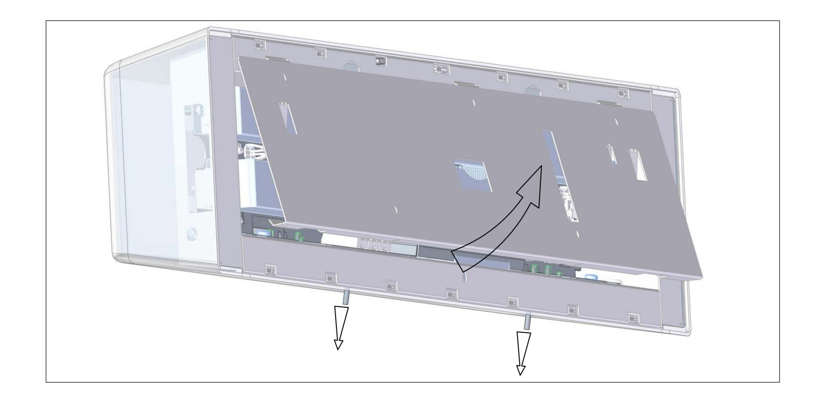
3. Mount the wall plate to the wall using all 5 x 5.0mm dia. mounting holes with suitable screw fixings. Note that the suspension cables will hang loose off the wall plate throughout this procedure.
