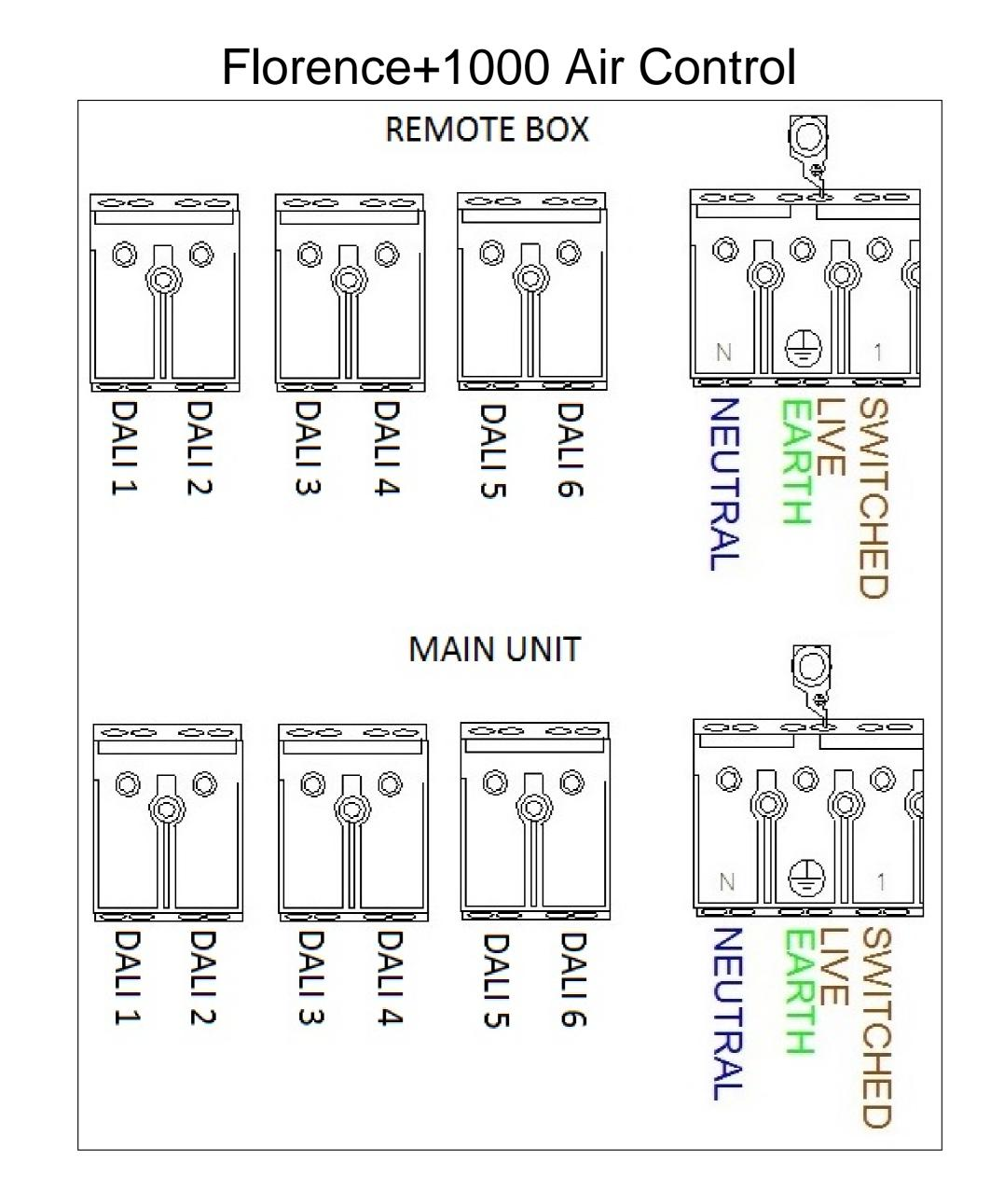
On the remote Aircontrol box the mains is to be looped out of the 3way block in the remote to the fitting. The Dali 1-6 is connected to the fitting Dali 1-6 with a 6 core cable as in Section 6. Max 1metre 1mm çable. See Section 6 for visual schematic.
