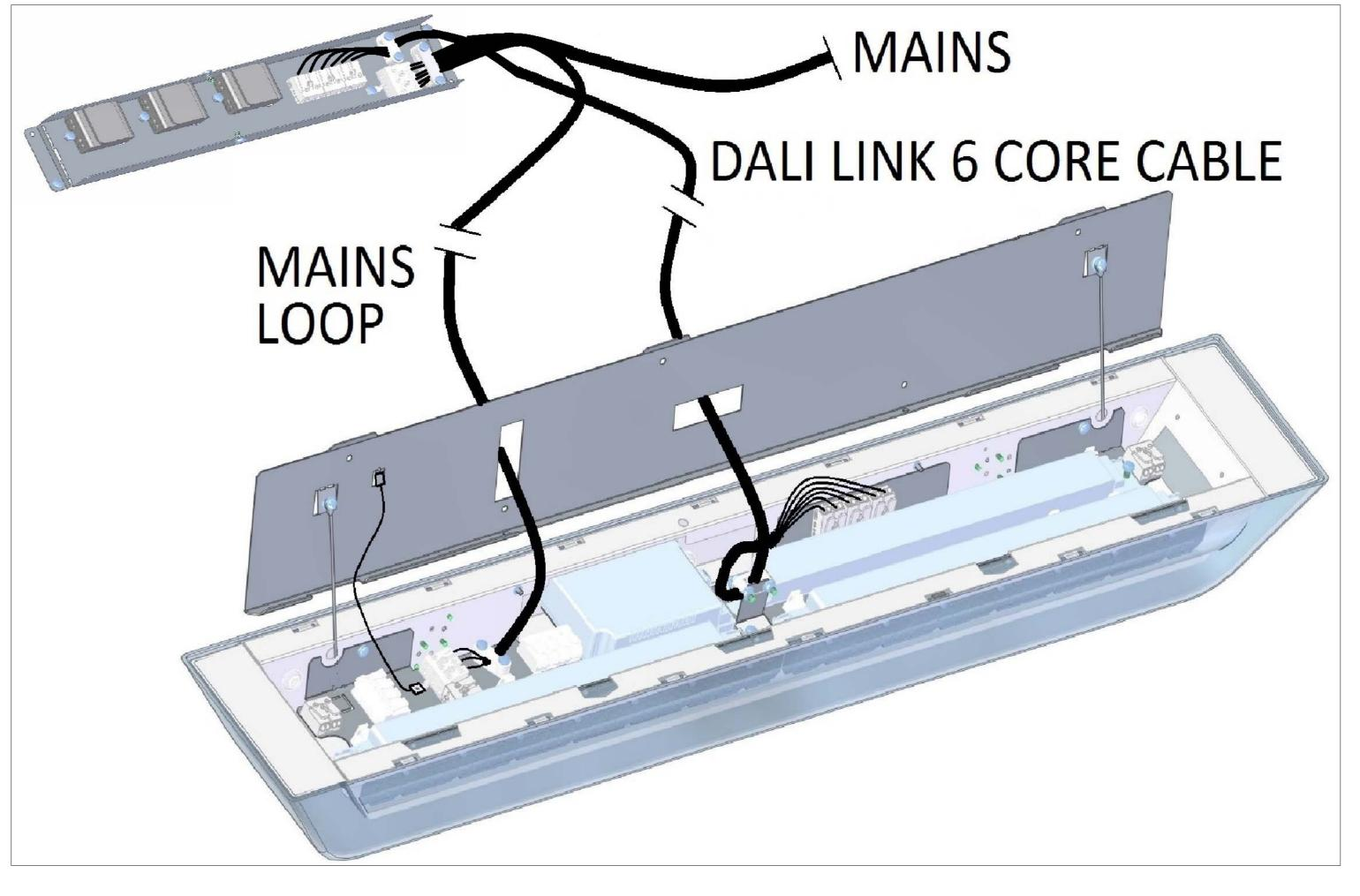
Mains Supply - 0.75mm<sup>2</sup> - 2.5mm<sup>2</sup>, Solid or Stranded mains rated.
