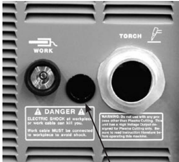
Pilot arc cable here.
