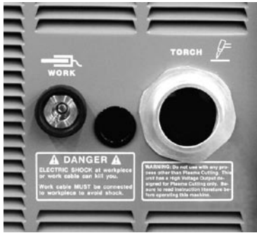
Thread service lines through bushing.
