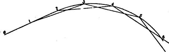
Fig. 1—Method of Measuring the Middle Ordinates of a Curve
