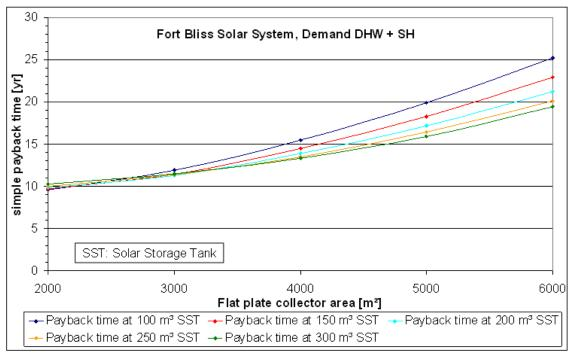
Figure B-28. Simple payback time depending on flat plate area, Fort Bliss, DHW and space heating.
