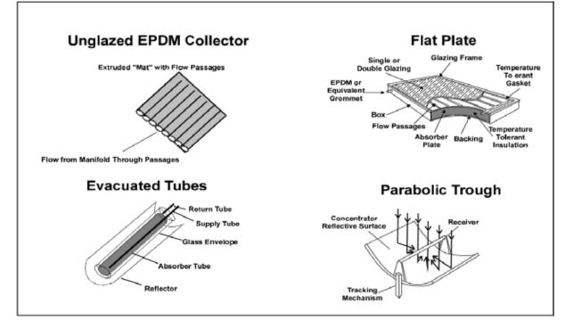
Figure 3.11. Types of solar thermal energy collectors.
