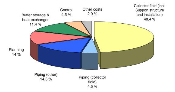
Figure 4.6. Distribution of costs for a large solar thermal system installation (Regenerative Energiesysteme).
