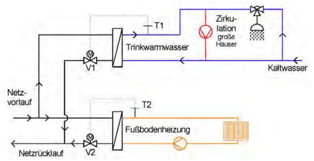
Figure A-44. Piping schematic of heat transfer stations in family houses (District heating Speyer "Old Slaughterhouse").
