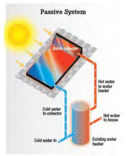
Figure 3.3. A simple passive solar water heating system with a batch collector.
