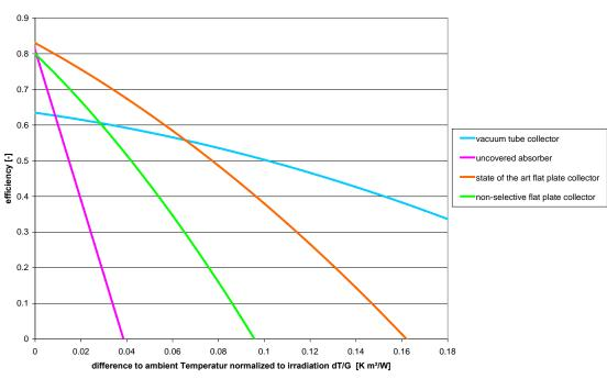
Efficiency for different solar collectors
