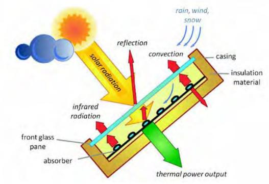
Figure 3.9. A Schematic of a flat plate collector (FPC) showing the heat gain and loss mechanisms that Play a role in determining the thermal efficiency of a collector (Regenerative Energiesysteme).
