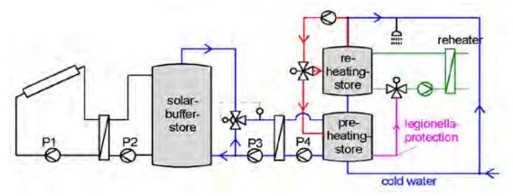
Figure A-39. Solar system for drinking water heating with pre-heating store and thermal disinfection for legionella-protection (with coverage of circulation losses).
