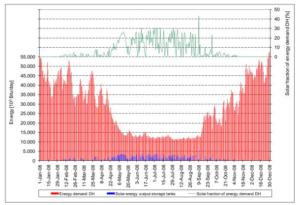
Figure A-71. Energy demand DH, solar energy output solar storage tanks and solar fraction of energy demand DH measured in 2008.
