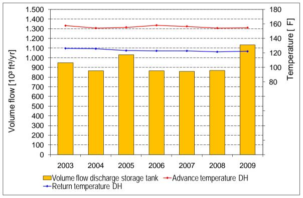
Figure A-59. Volume flow discharge solar storage tank, advance and return temperature DH.
