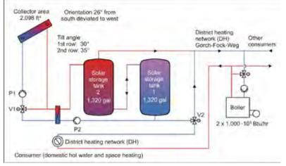
Figure A-49. Highly simplified schematics of the solar system, solar storage tanks arrangement and the integration in the district heating network (DH).
