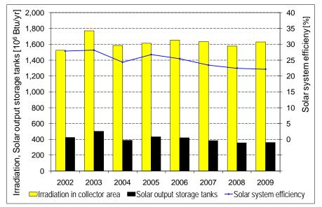
Figure A-66. Irradiation in collector area, solar energy output from solar storage tanks and solar system efficiency.
