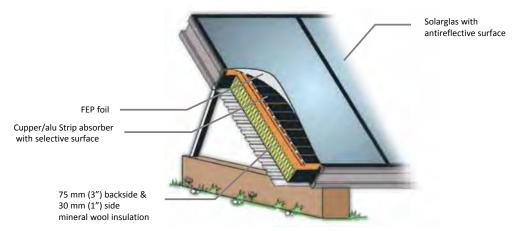
Figure A-35. Cross section of the ARCON HT collector.
