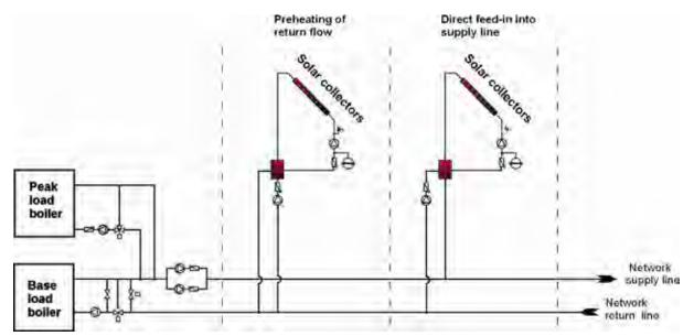
Figure 3.26. Solar supported district heating network with direct interconnection of a central solar thermal system.
