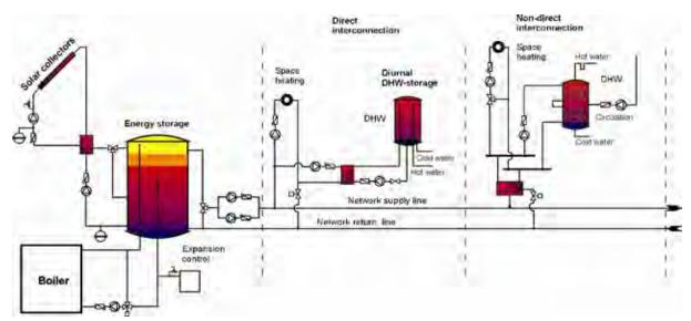
Figure 3.22. Solar supported two-pipe network with centralized energy storage and decentralized domestic hot water storages.
