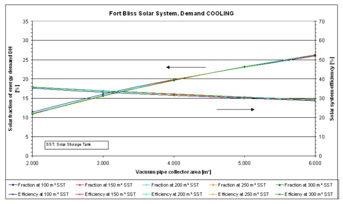
Figure B-7. Solar fraction and solar efficiency depending on vacuum pipe area, Fort Bliss, cooling.
