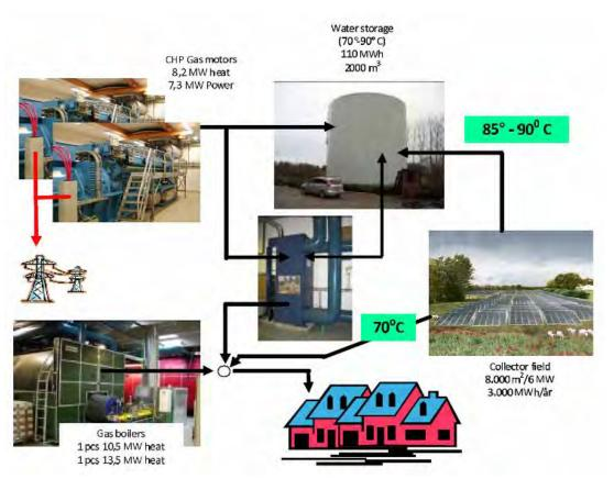
Figure A-34. Overview of the District Heating System of Brædstrup.
