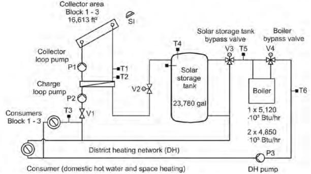
Figure A-84. Highly simplified schematics showing the positioning of the control sensors.
