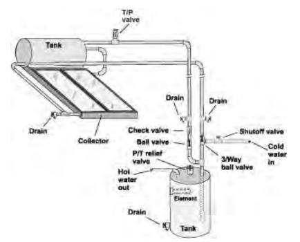
Figure 3.4. Schematic of a typical thermosiphon system.
