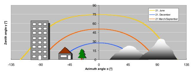
Figure 2.8. Influence of structures on shading of incoming solar radiation. Height and distance both need to be taken into account.
