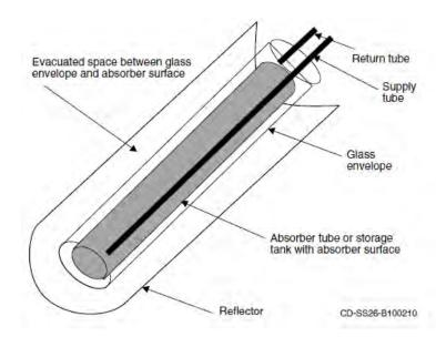
Figure 3.14. Evacuated-tube collector.
