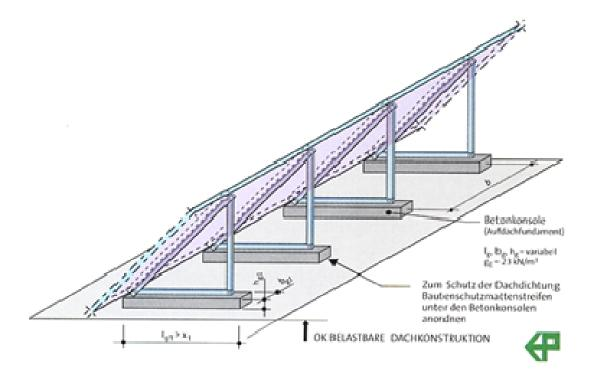
Figure 5.7. Collectors mounted on concrete slab.
