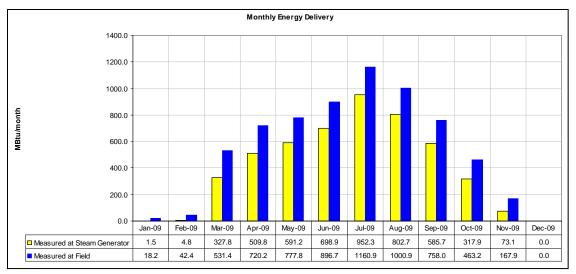
Figure A-131. Chart showing the monthly energy delivery of the solar water heating system at the SunChips<sup>®</sup> factory in Modesto, CA, which is owned by Frito Lay. The annual energy collected was 14,600 MB tu/yr/sq ft in 2009.
