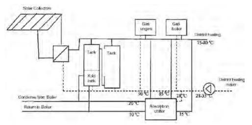
Figure A-23. Diagram of district heating system.
