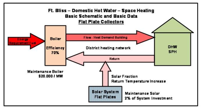
Figure B-29. Basic schematic – Fort Bliss – DHW / SPH – flat plate collectors.
