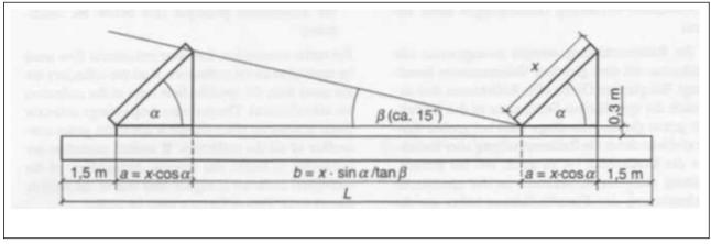
Figure 5.5. Spacing between collector rows.
