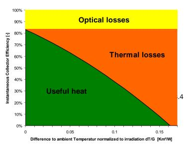
Figure 3.18. Typical solar collector efficiency curve with losses and useful heat indicated.
