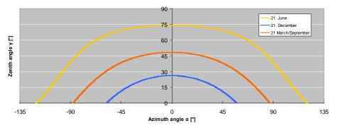
Figure 2.4. Path of the sun for latitude = 38° 53" (Washington, DC) relative to a horizontal plane.
