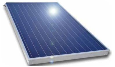
Figure 3.13. Flat plate collector with selective coating on the absorber. The parallel lines indicate where the riser tubes are connected to the absorber by ultra-sonic welding.
