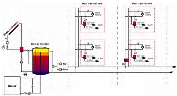
Figure 3.21. Solar supported two-pipe network with centralized energy storage and decentralized heat transfer units.
