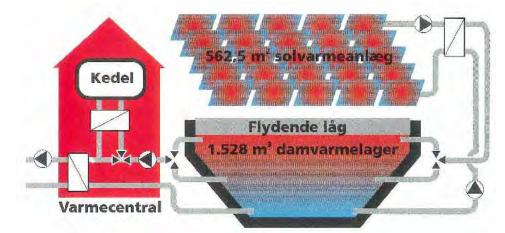
Figure A-29. Diagram of the heating system.
