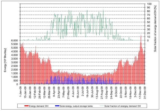
Figure A-78. Energy demand DH, energy output solar system and solar fraction of total energy demand DH measured in 2009.
