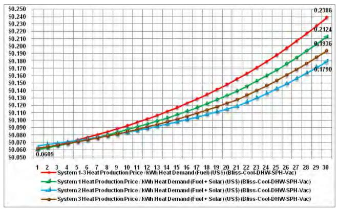
Figure B-26. Energy cost - Fort Bliss – DHW / SPH / cooling – vacuum tube collectors.
