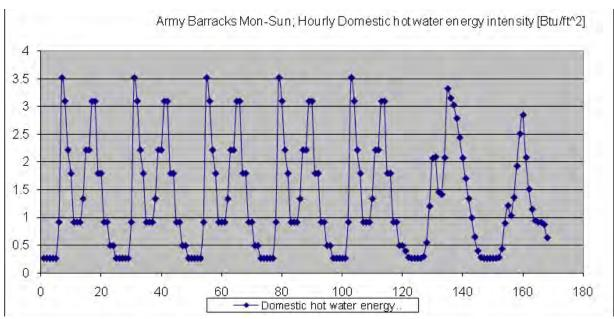
Figure 4.2. Weekly barracks domestic hot water heating profile, Btu/sq ft by hour.
