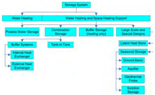
Figure 3.28. Overview of storage system types and their application.
