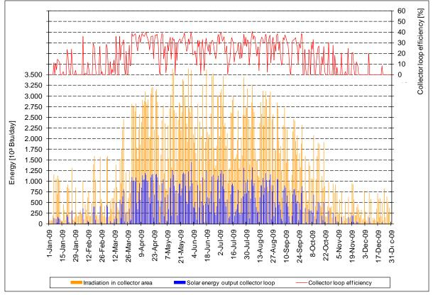
Figure A-76. Irradiation, energy output, and efficiency collector loop in 2009, daily data solution.
