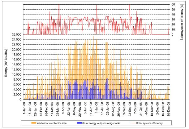
Figure A-60. Irradiation, energy output solar storage tank and efficiency solar system in 2008, daily data solution.
