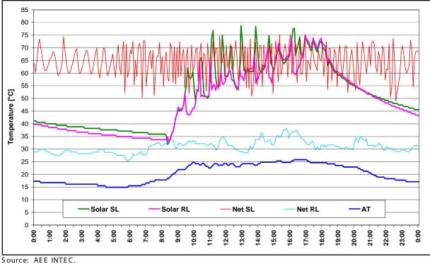
Figure A-9. Temperatures of the solar loop and the distribution grid in July 2<sup>nd</sup> 2001, Gneis-Moos.
