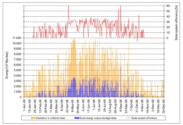
Figure A-69. Irradiation in collector area, solar energy output from solar storage tanks, and solar system efficiency in 2008, daily data solution.
