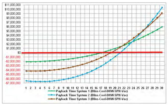
Figure B-25. Payback time - Fort Bliss – DHW / SPH / cooling – vacuum tube collectors.
