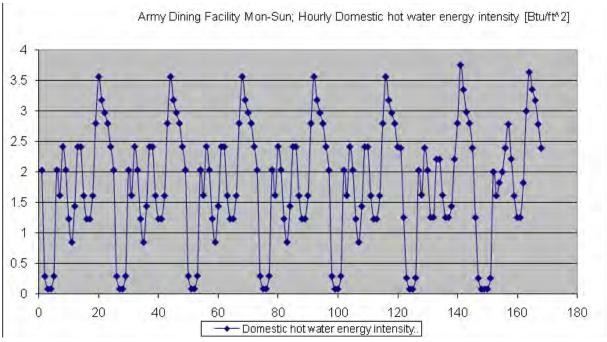
Figure 4.3. Weekly domestic hot water heating profile, Btu/sq ft by hour for a dining facility.
