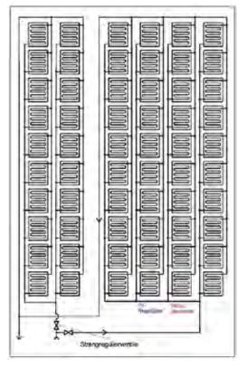
Figure A-37. Piping schematic of the fassade collector field (Apartment House Frankfurt).
