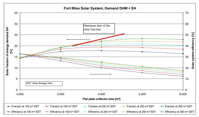
Figure B-13. Solar fraction and solar efficiency depending on flat plate area, Fort Bliss, DHW and space heating.
