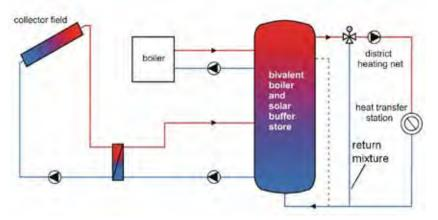
Figure A-43. Heating net with four-pipe boiler reheating inside buffer store.
