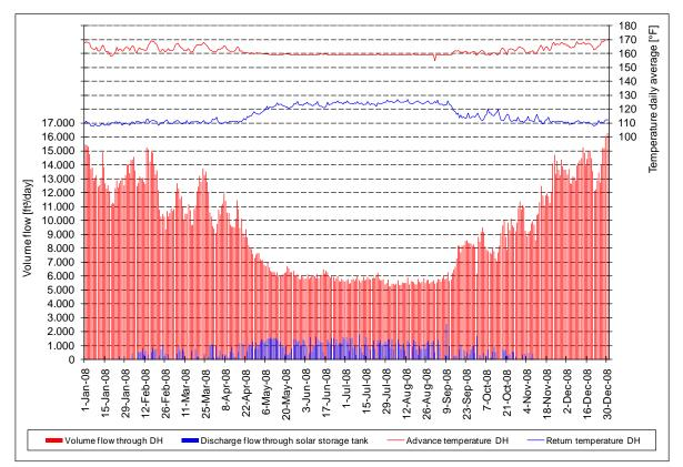
Figure A-72. Volume flow DH, discharge flow through solar storage tanks and temperatures DH.
