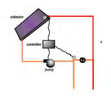
Figure 3.8. Schematic of a recirculating loop system. These systems require well insulated collectors such as evacuated tube to provide protection for freezing and overheating.
