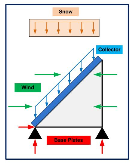
Figure 5.2. Forces on solar collector that determine structural requirements.
