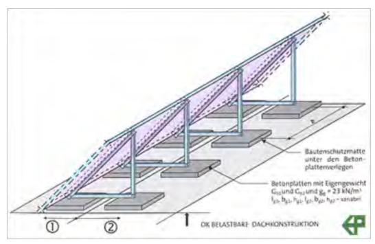
Figure 5.8. Roof support construction example.
