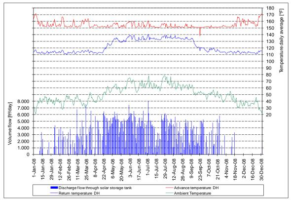
Figure A-62. Discharge flow through solar storage tank and temperatures DH in 2008.
