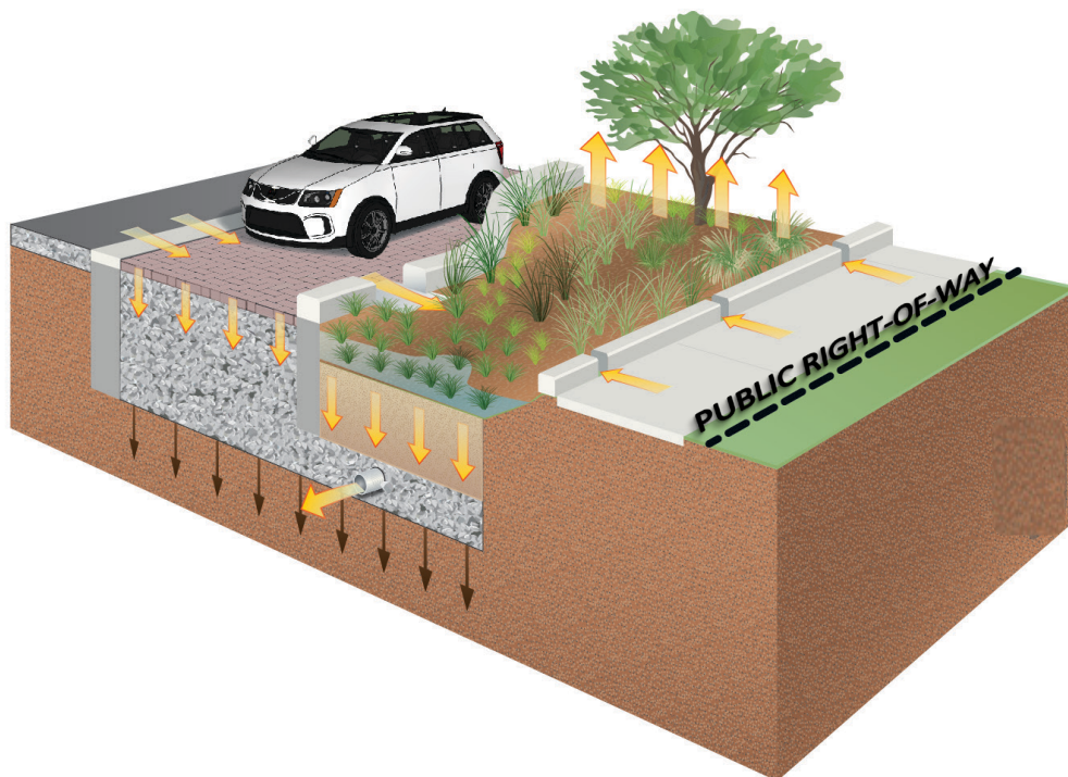
Figure A-1 Conceptual schematic of ROW BMPs with an underdrain (Arrows indicate water path ways)
