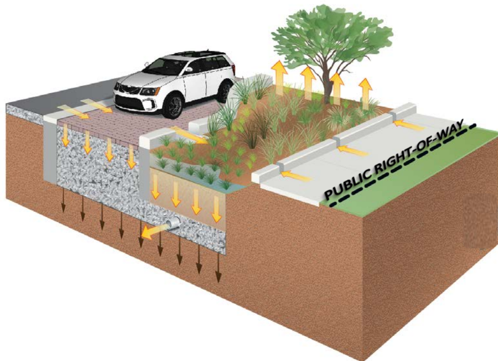
Figure 0-1 Conceptual schematic of ROW BMPs with an underdrain (Arrows indicate water path ways)
