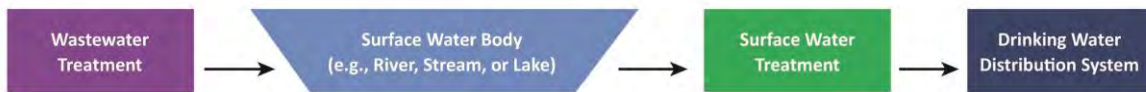
Figure 1-3: Schematic of unplanned ( de facto ) potable reuse, which involves the discharge of treated wastewater effluent from one community into a surface water body that is used as a source of drinking water supply for another community. Depending upon the location and local requirements, wastewater treatment could vary, but for the most part freshwater discharges in California include secondary treatment followed by filtration and disinfection. Surface water treatment includes filtration and disinfection.
