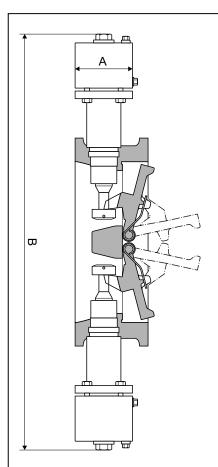
BB with patented adjustable dampers, DN 200 – 500.
