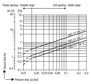
Curve 1: SBO 31 DN 3/4" Curve 2: SBO 31 DN 1"
