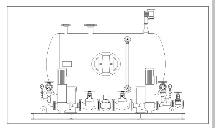
Condensate receiver tank of cylindrical design type SD L (S) with high-pressure centrifugal pump(s) installed next to the tank L = horizontal design; S = vertical design
