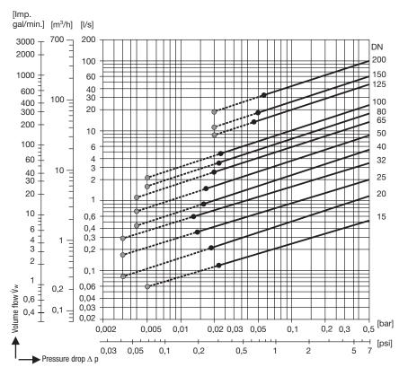
Required minimum volume flow W for equipment without spring installed in vertical pipes with upward flow.
