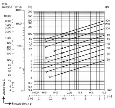
Required minimum volume flow V<sub>W</sub> for equipment without spring installed in vertical pipes with upward flow.
