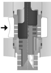
Throttling unit A1/A2 with 4-stage expansion
