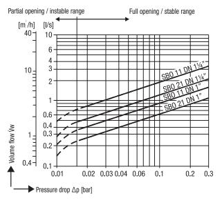
Curve 1: SBO 21 DN 1" Curve 2: SBO 11 DN 1"
