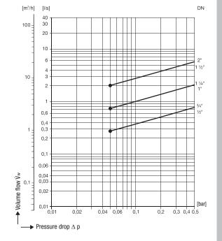
Required minimum volume flow  $\dot{V}_W$  for equipment without spring installed in vertical pipes with upward flow (only RK 70, RK 71).
