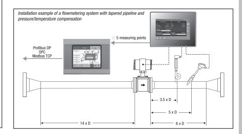
Steam-flow measurement system for constant saturated steam pressure
