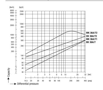
The chart shows the discharge capacity of hot condensate
