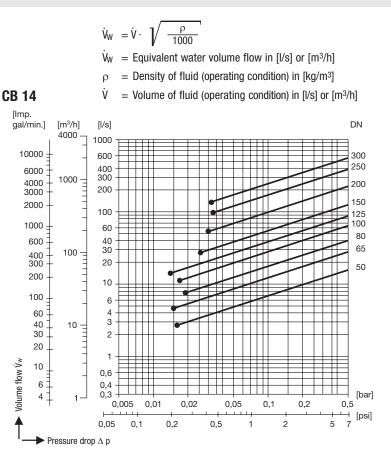
• Required minimum volume flow  $\dot{V}_W$  for equipment installed in horizontal pipes.
