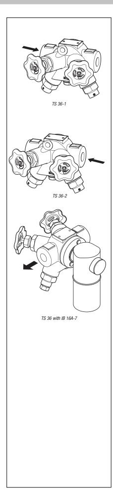
The compact-type Trap Station TS 36 features additional test and shut-off functions and is a more convenient alternative to the simpler connector units UC 36 and UCY 36.
