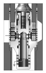
Radial stage nozzle with tandem shut-off for ZK 213
