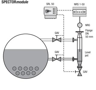
Accessories for high-integrity level controls fitted in an external level control pot
