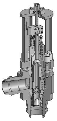
3-stage expansion with balanced pressure for ZK 613
