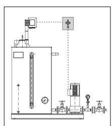
Condensate tank of rectangular design type SDR A with high-pressure centrifugal pump(s) installed next to the tank
