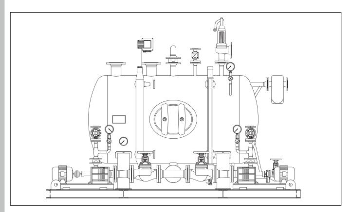
Condensate receiver tank of cylindrical design type SD L (S) with horizontal-type centrifugal pump(s) installed next to the tank L = horizontal design; S = vertical design
