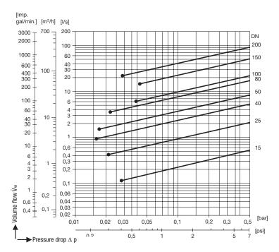
Required minimum volume flow V<sub>W</sub> for equipment with standard spring and horizontal flow.
