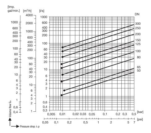
Required minimum volume flow W for equipment installed in horizontal pipes.
