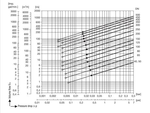
• Required minimum volume flow  $\dot{V}_W$  for equipment without spring installed in vertical pipes with upward flow.
