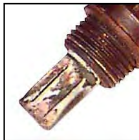
Ethylene Glycol (Antifreeze) Contamination
