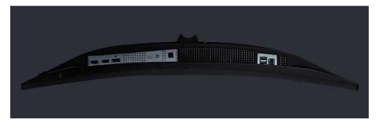
The XG3240C integrated interface includes:  $2 \times \text{HDMI}$  (2.0),  $1 \times \text{DisplayPort}$ ,  $5 \times \text{USB}$  (1 up, 4 down) and  $2 \times 6 \text{W}$  speakers
