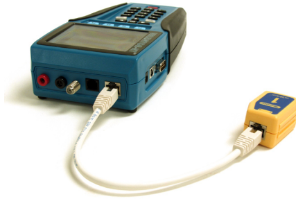
Figure 7. Wiremapper Remote #1 Connected to Validator-NT
