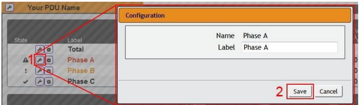
Figure 3-17 Phase and Circuit Labeling
