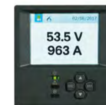
Home page of the DMU showing total voltage and current.
