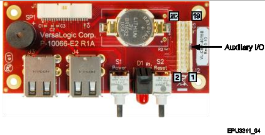
Figure 28. Location and Pin Orientation of Auxiliary I/O Connector
