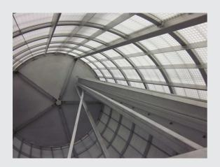
Hydrotech's patented filter panels improve the hydraulic capacity and offers better lifting properties. The drum is constructed in sections, each with up to 5 filter panels depending on diameter. This makes it easy to design a solution according to your specific requirements.
