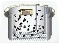
The ANITA Mox effluent screens provide a positive barrier to loss of anammox bacteria, since they keep the media and biofilm in the reactor.
