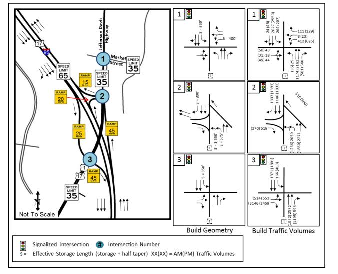
Figure 10. Build Traffic Volumes and Geometry
