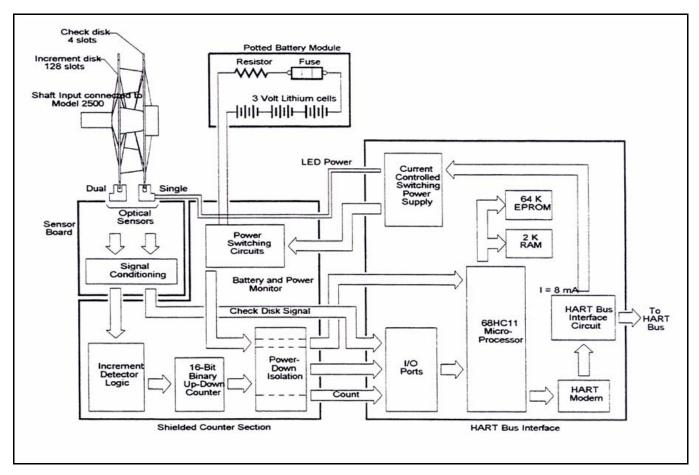
Figure 6-1: 4110 HLE Block Diagram
