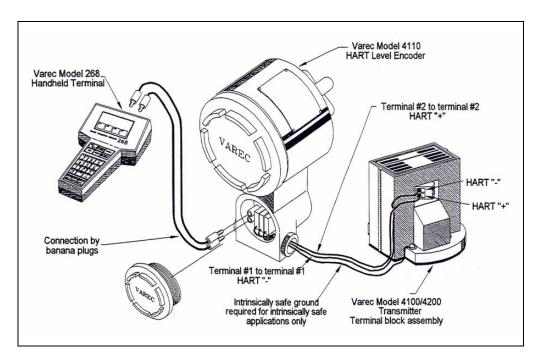
Figure 2-4: 4110 HLE Wiring Connections
