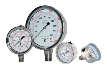
WGI Elite series stainless steel pressure gauges have a 304 stainless steel case for use in harsh or corrosive environments. These gauges are liquid filled for significant cushioning and pulsation dampening which reduces pointer flutter and internal damage. Industries suited for these gauges include oil and gas equipment, refineries, hydraulic equipment, agricultural equipment, pressure washers, pumps, compressors and process systems.
