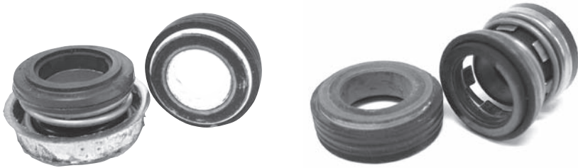
PTFE or Silicone Based Lubricants Damage Seals
