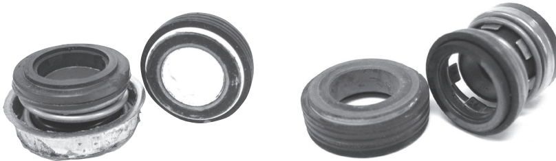
PTFE or Silicone Based Lubricants Damage Seals
