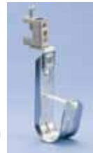
CAT12 J-Hook • Accepts up to 16 4-pair UTP CAT 5e or 2-strand fiber optic cable, or 10 CAT 6 - 3/4" dia
