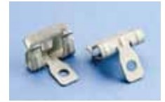
4H24 Hammer-On Flange Clip, Side Mount • Provides a "portable" hole • Fits most beams and bulb tees • Installs with just a hammer
