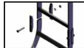
12. BUTT SPLICES ICCMSLEBSK Joins ladder rack runway at ends 2 each
