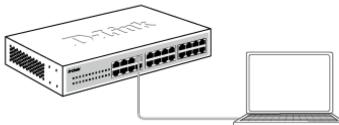
Figure 4-1 – Connecting to a DGS-1100 MP/MPP Series switch
