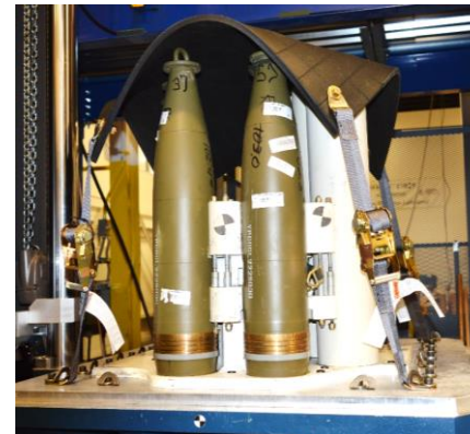
Ammo Rack Retention Test
