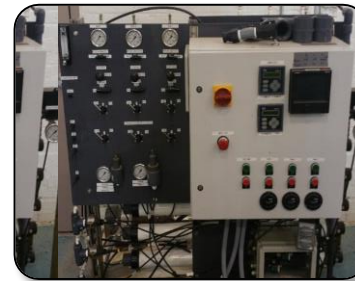
RO Element Test Stand
