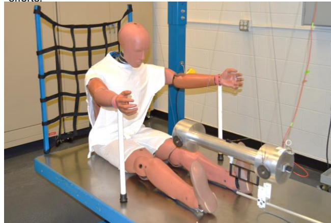
Thorax Impact Test Device
