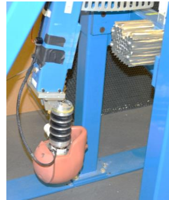
Neck Pendulum Test Device
