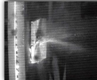
High speed cameras are used to capture frame-by-frame ballistic impact data on targets
