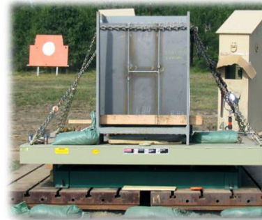
Target setup for weld evaluation testing
