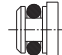
plug for 3/2 valve mounting CP-112 for G1/8, CP-9112 for G1/4 material: aluminium
