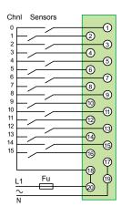
L1-N voltage: 24 V  $\sim$ , BMX DAI 1602 48 V  $\sim$ , BMX DAI 1603 100/120 V  $\sim$ , BMX DAI 1604 Fu: 0.5 A fast-blow fuse
