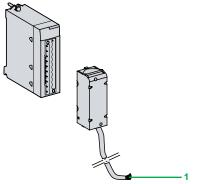
BMX FTW •01S cordset (with 20-way removable terminal block at one end and flying leads at the other)
