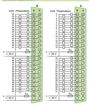
BMX DDO 3202K: Connector A (outputs I0...I31)
