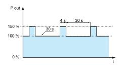
The **ABL 8RPS/RPM/WPS** Universal range of Phaseo® power supplies has a power reserve, allowing them to supply the application with energy up to 1.5 times the nominal current at the intervals illustrated by the graph on the left.
