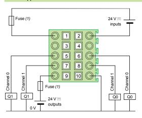
A fast-blow fuse to protect the module electronics in the event of reversed polarity of the power supplies on I/O.
