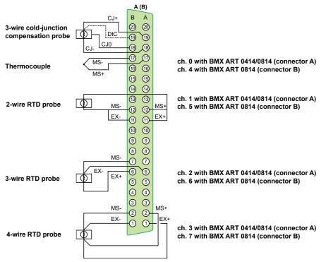
MS+: Input + RTD probe or thermocouple MS-: Input - RTD probe or thermocouple EX+: Output + RTD probe current generator EX-: Output - RTD probe current generator
