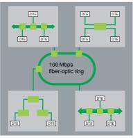
Switches are used to increase the limits of architectures based on hubs or transceivers by separating collision domains.
