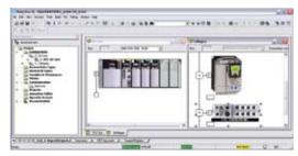
Graphical configuration of devices on CANopen bus
