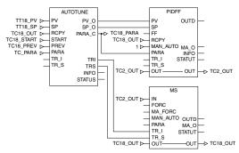
Example: PID controller with MS manual control
