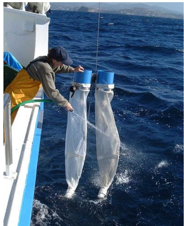
Plankton sampling using a Bongo Net. © María Luz Fernández de Puellas
