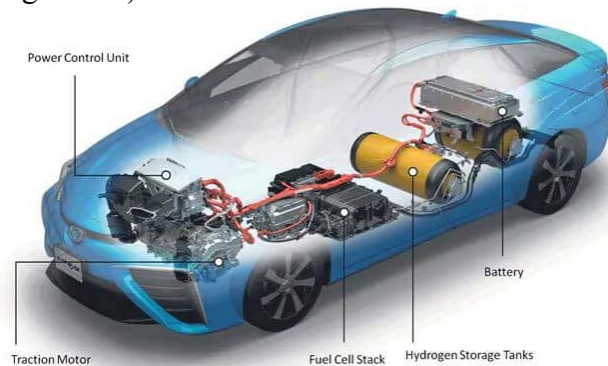
Figure 6.7 Internal Working of a Typical Fuel Cell Vehicle [Spiegel, 2019]
