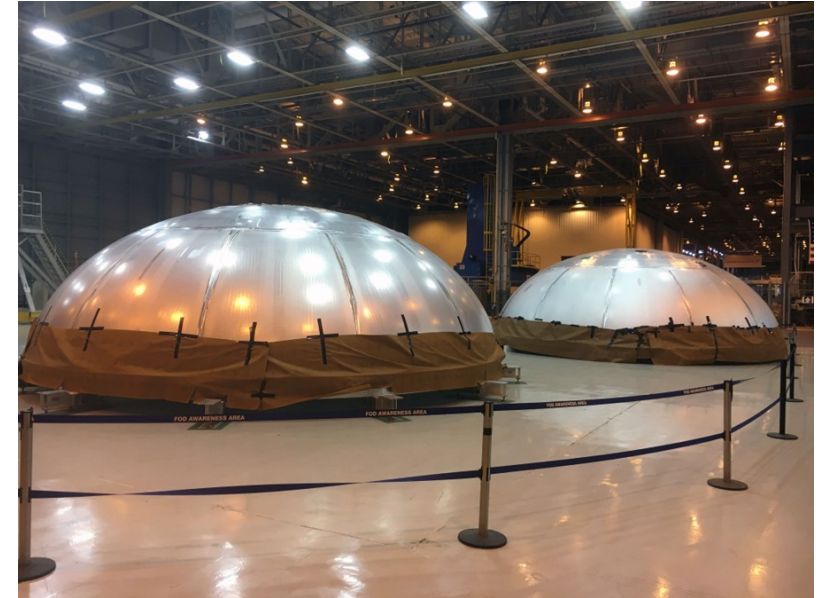
Two fuel tank domes were recently finished for the SLS rocket. One is a qualification article and the other is the actual flight article for the first mission
