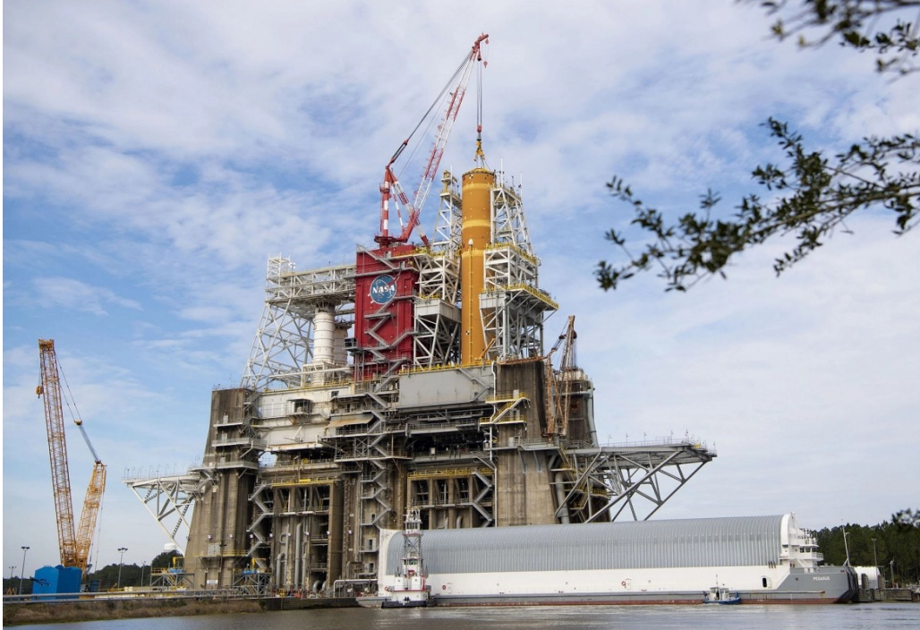
SLS Core Stage is removed from Pegasus barge and installed in the B-2 position at the B Test Stand at the Stennis Space Center (SSC) in Mississippi
