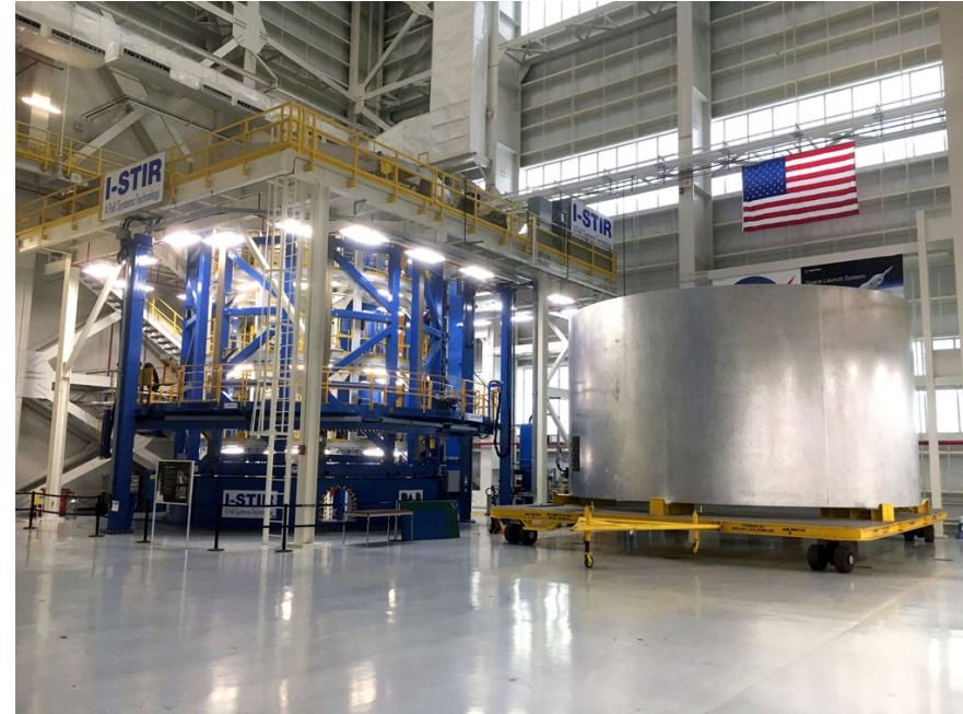
The Vertical Weld Center tool used to fabricate barrel segments for the SLS liquid hydrogen and oxygen core stage tanks via vertical friction stir welding operations To the right of the welder is the weld confidence barrel
