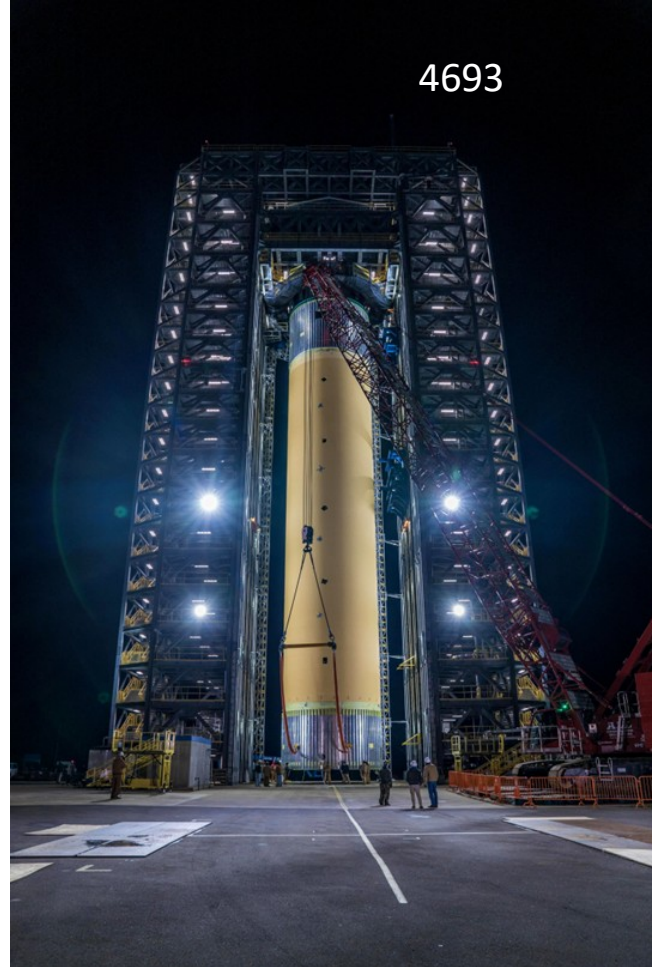
The SLS liquid hydrogen tank structural test article in a cage-like test stand at MSFC
