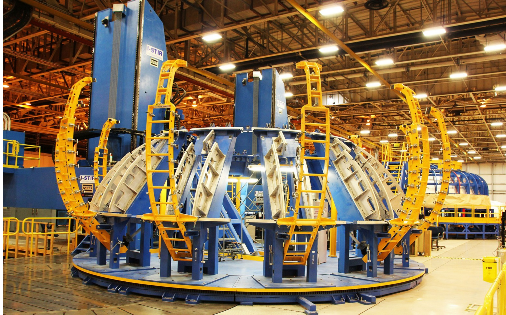
The Gore Weld Tool (foreground) and Circumferential Dome Weld Tool (background) used to fabricate dome segments for the SLS liquid hydrogen and oxygen core stage tanks via vertical friction stir welding operations
