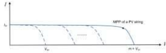
Figure 4. I-V curve of a PV string with m modules in series (Zhao,2010)
