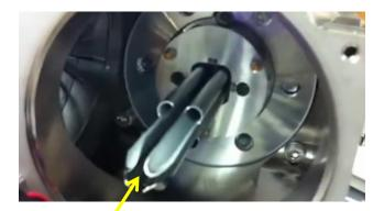
View of the first set of quadrupoles (designated as **Q0** in the diagram on page 1) with the orifice plate removed. It is here that the entrance potential (**EP**) is applied.
