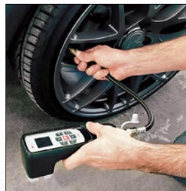
Checking air pressure
