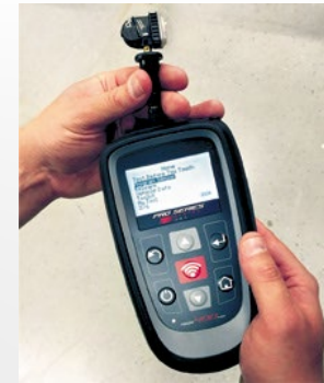
Programming a replacement sensor
