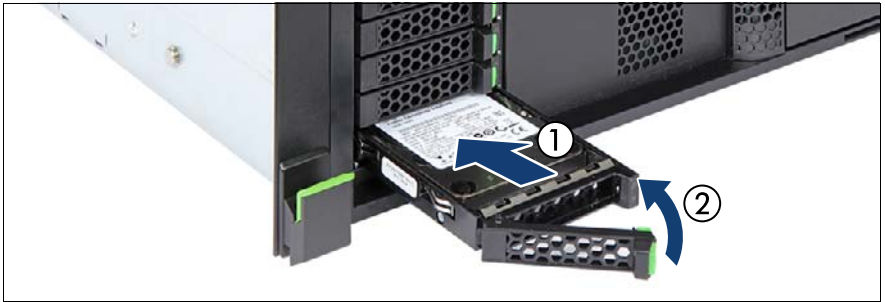
Figure 25: Installing the 2.5-inch HDD/SSD module
