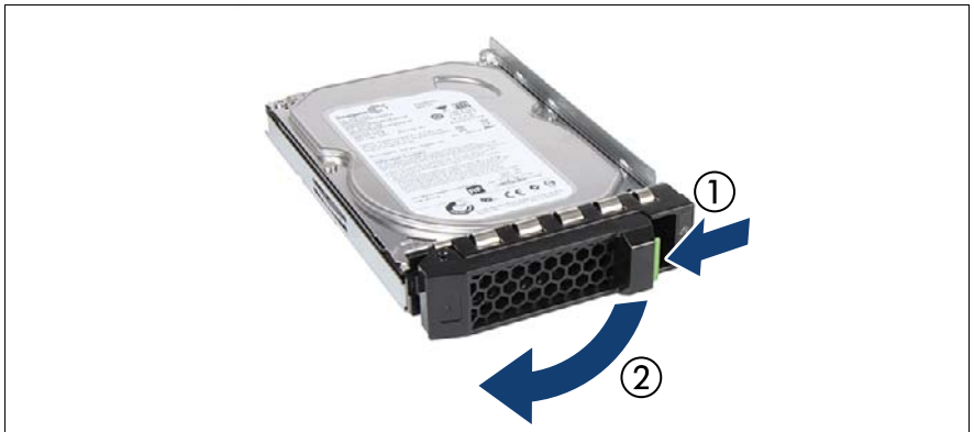
Figure 21: Opening the 3.5-inch HDD module locking lever
