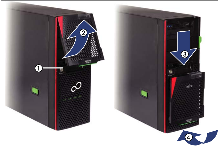
Figure 18: Removing the accessible drive bay cover
