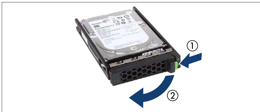
Figure 24: Opening the 2.5-inch HDD/SSD module locking lever
