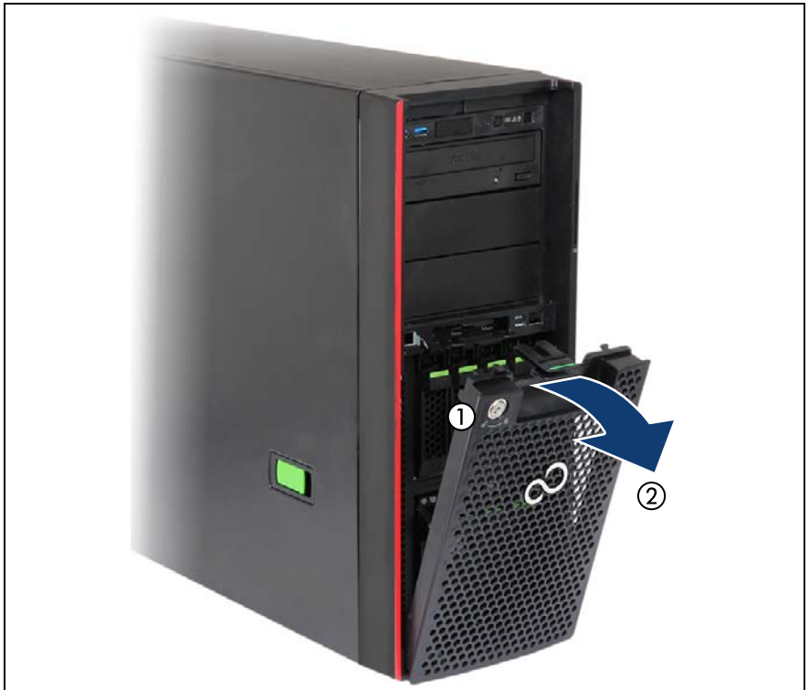
Figure 19: Removing the HDD bay cover
