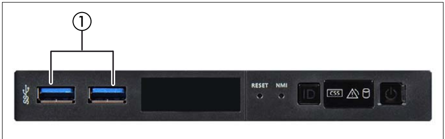
Figure 5: Connectors on the front panel
