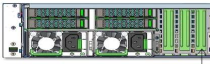
Slot 7 to use for 4x2.5" rear solutions separate
