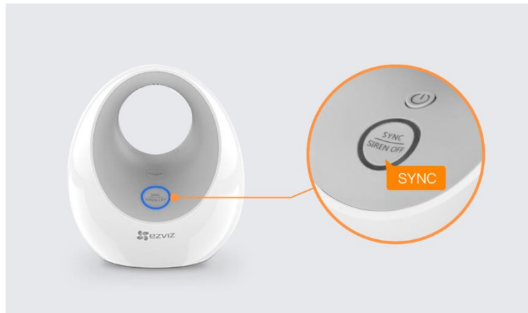
Figure 5-8 Press the SYNC Button
